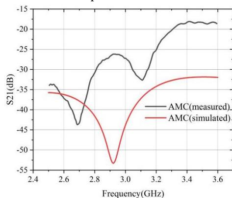
(b) Isolation between two ports of dual-polarized crossed dipole with AMC surface
