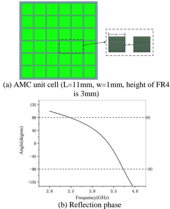
Fig. 5. AMC unit cell and reflection phase.
