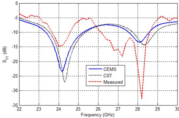
Fig. 3. Simulated and measured  $S_{11}$  of the antenna.
