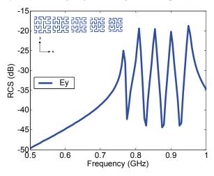
Fig. 7. Expanded (zoomed in) E<sub>y</sub> frequency signature for 5-element Hilbert RFID tag, shown in inset.
