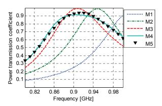
Fig. 7. Power transmission coefficient with stray capacitance value  $C_s$ =0.2 pF.
