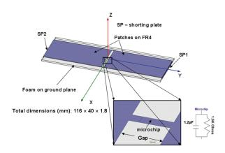
Fig. 2. Design of the RFID tag antenna.
