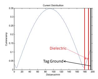
Fig. 5. Current distribution along longer coax fed for the PIFA tag.
