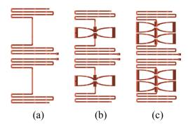
Fig. 2. (a) Layout of the omega structure with no deformed omega elements (N = 0); (b) layout of the omega structure with two deformed omega elements (N = 2); (c) layout of the omega structure with four deformed omega elements (N = 4).
