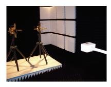
Fig. 4. Measuring the tag in an anechoic chamber.
