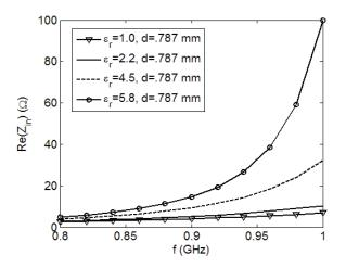
Fig. 6. Input resistance of the omega structure for various values of  $\epsilon_{\text{r}}$ .
