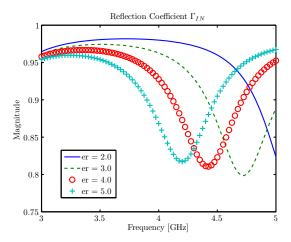
Fig. 4. Magnitude of  $\Gamma_{IN}$  for  $\epsilon_{r2}=2, 3, 4$  and 5 calculated from the signal flow graph.
