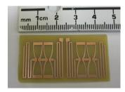
Fig. 3. Omega structure-based meander-line RFID antenna (s = 0.5 mm, k = 1.0 mm, m = 42.2 mm, a = 5.0 mm, p = 0.86 mm,  $\delta$  = 4.0 mm,  $\Delta$  = 18.8 mm,  $\epsilon$ <sub>r</sub> = 3.75 (measured) and d = 0.787 mm).
