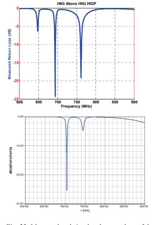
Fig. 23. Measured and simulated return loss of the fabricated Hilbert antenna above Hilbert high-impedance ground-plane.
