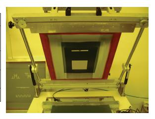
Fig. 5. Placement of the stencil screen onto the screen printing machine.
