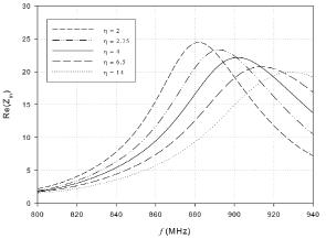
Fig. 4. Real part of the antenna input impedance for different values of  $\eta = l_y / l_a$ .
