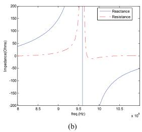
Fig. 1. Nonphysical results obtained when a short coax used to feed a PIFA tag: (a) Geometry of short coax feeding a PIFA tag; (b) Input impedance.
