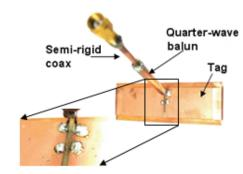
Fig. 7. Quarter-wave balun soldered to the prototype tag.
