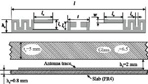
Fig. 1. UHF tag antenna layout and simulation model.
