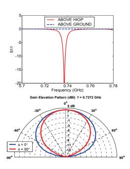
Fig. 20. Hilbert RFID tag utilizing a Hilbert HIGP (AMC) for enhanced radiation performance.
