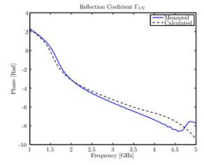
Fig. 10. Comparison between measured and calculated phase of reflection coefficient ( $\angle\Gamma_{in}$ ).
