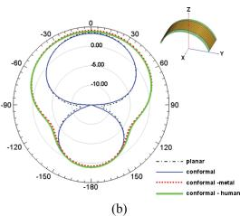
Fig. 13. Comparison between planar tag, conformal tag, conformal tag on metal and conformal tag on human arm. (a) Radiation pattern in the xz-plane ( $\varphi = 0^{\circ}$ ). (b) Radiation pattern in the yz-plane ( $\varphi = 90^{\circ}$ ).
