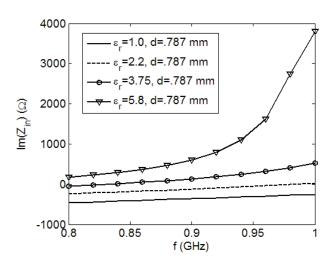
Fig. 18. Input reactance of the SRR structure for various values of  $\varepsilon_r$ .
