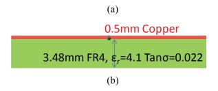
Fig. 3. Geometry of mender tag: (a) Top view; (b) Side view.
