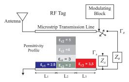
Fig. 3. The transmission line model of the RF tag, illustrating four changing permittivity profiles of the center well of the REMS sensor.
