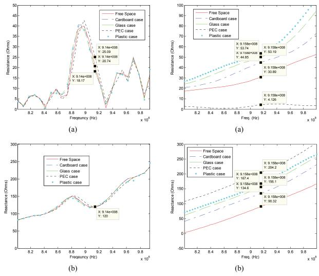
Fig. 6. Input impedance of PIFA: (a) Resistance; (b) Reactance.
