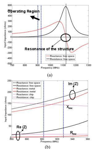
Fig. 4. Simulated input impedance of the antenna. (a) In free space. (b) In free space and on a 250mm x 250mm x 2mm copper plate. The 902–928 MHz band is marked by two vertical lines.
