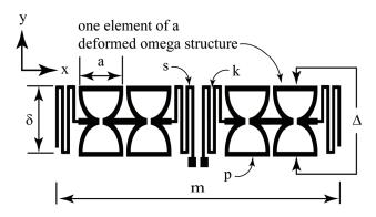
Fig. 1. Deformed omega structure-based meander-line RFID antenna dimensions [28].
