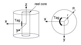
Fig. 3. Tag antenna placement on the reel core.
