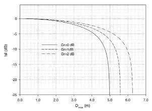
Fig. 3. Return loss as a function of the maximum achievable reading range for different tag antenna gain ( $P_{th} = -13 \text{ dBm}$ , p = 0.5, f = 867 MHz,  $P_{eirp} = 35.16 \text{ dBm}$ ).
