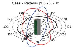
Fig. 11. Scattering Patterns of the Peano-curve RF tag on a paper roll of 37.5mm radius at 0.76GHz.
