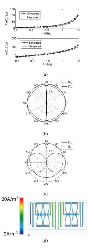
Fig. 5. (a) Measured and simulated input impedance of a deformed omega structure-based meander-line RFID antenna; (b) simulated pattern in the y-z plane; (c) simulated pattern in the x-z plane; (d) simulated surface current at 920 MHz.
