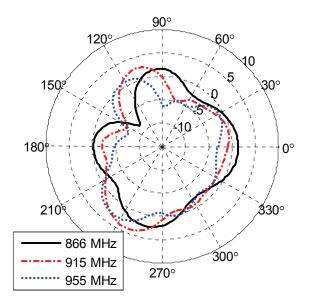
Fig. 9. Directivity [dBi] of the paper reel C-tag, from model M5 in the xy-plane (as in Fig. 3) at three different frequencies.
