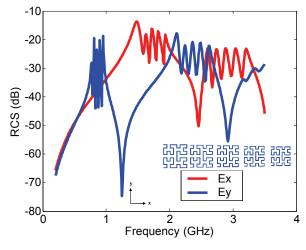
Fig. 6. Frequency signature for 5-element Hilbert RFID tag (inset) for both polarization excitations.
