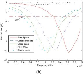
Fig. 8. Return Loss Charcteristics of two tag antennas: (a) PIFA; (b) Meander tag.
