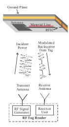
Fig. 1. Components of a REMS Sensor.
