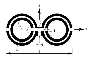
Fig. 15. Dimensions of the split-ring resonator-based RFID antenna.
