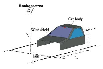
Fig. 8. Simulated single-lane vehicle identification scenario.
