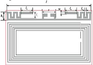
Fig. 2. UHF-HF integrated transponder layout.
