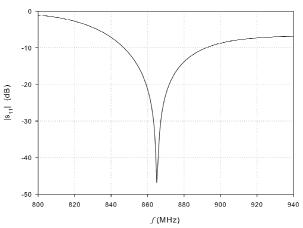
Fig. 6. Antenna input reflection coefficient.
