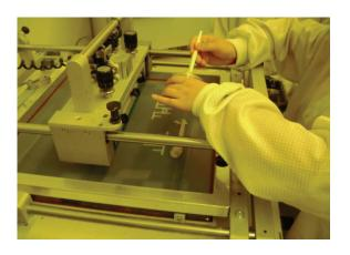
Fig. 7. Transferring the squeegee across the stencil to imprint the design on the substrate.
