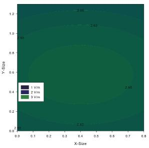
Fig. 9. Electric field intensity at the observation plane without the car body.
