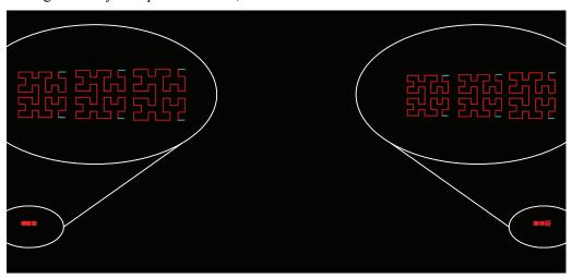
Fig. 16. Two separate Hilbert curve RFID tags.
