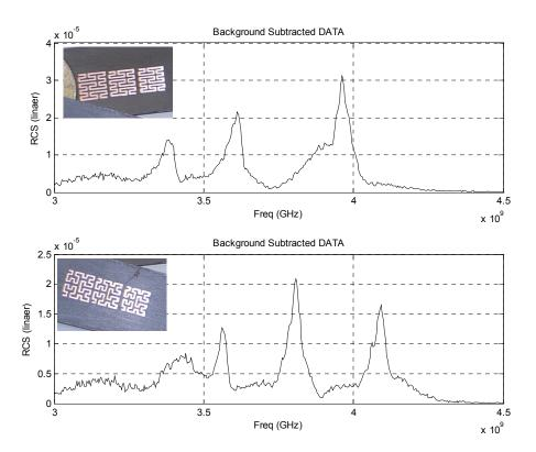
Fig. 13. Measured frequency signature for 3-element Peano and Hilbert RFID tags.
