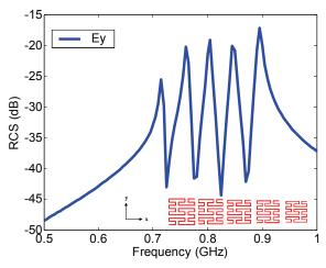
Fig. 5. Expanded (zoomed in) E<sub>y</sub> frequency signature for 5-element Peano RFID tag, shown in inset.
