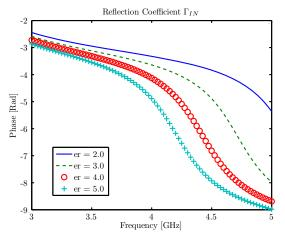
Fig. 5. Phase of  $\Gamma_{IN}$  for  $\epsilon_{r2}=2, 3, 4$  and 5 calculated from the signal flow graph.
