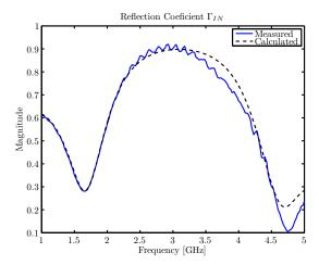
Fig. 9. Comparison between magnitude of measured and calculated reflection coefficient ( $|\Gamma_{in}|$ ).
