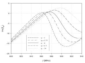
Fig. 5. Imaginary part of the antenna input impedance for different values of  $\eta = l_v / l_a$ .
