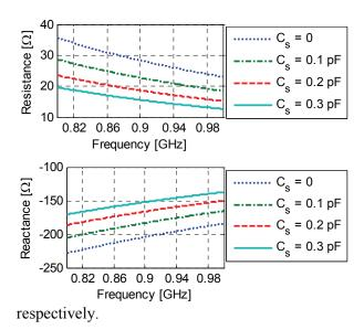
Fig. 5. The effect of the stray capacitance to the input impedance of the IC chip.
