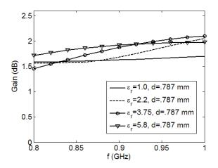
Fig. 19. Gain of the SRR structure for various values of  $\varepsilon_r$ .
