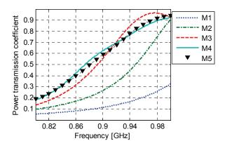
Fig. 6. Power transmission coefficient with an ideal antenna-chip connection ( $C_s$ =0).
