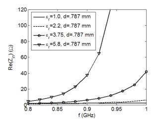
Fig. 17. Input resistance of the SRR structure for various values of  $\varepsilon_r$ .
