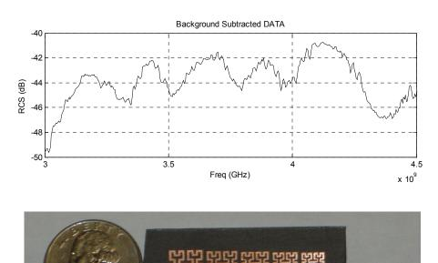
Fig. 14. Measured frequency signature for 5-element Hilbert RFID tag.
