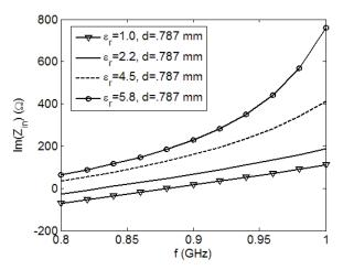
Fig. 7. Input reactance of the omega structure for various values of  $\varepsilon_r$ .
