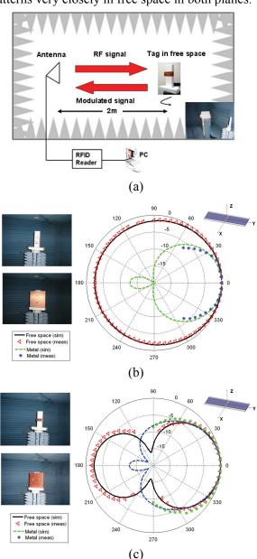
Fig. 9. (a) Radiation pattern measurement setup. (b) Normalized measured and simulated radiation pattern in the XZ-plane ( $\Phi = 0^{\circ}$ ). (c) Normalized measured and simulated radiation pattern in the YZ-plane ( $\Phi = 90^{\circ}$ ). The antenna is in free space and on a 250 mm × 250mm x 2mm copper plate. The scale is in dB.
