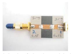
Fig. 8. Snapshot of microstrip transmission line setup for experimental measurements.
