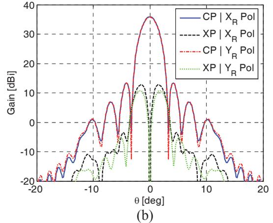
Fig. 2. Radiation pattern of the boresight beam. Main cuts in elevation (a) and azimuth(b).
