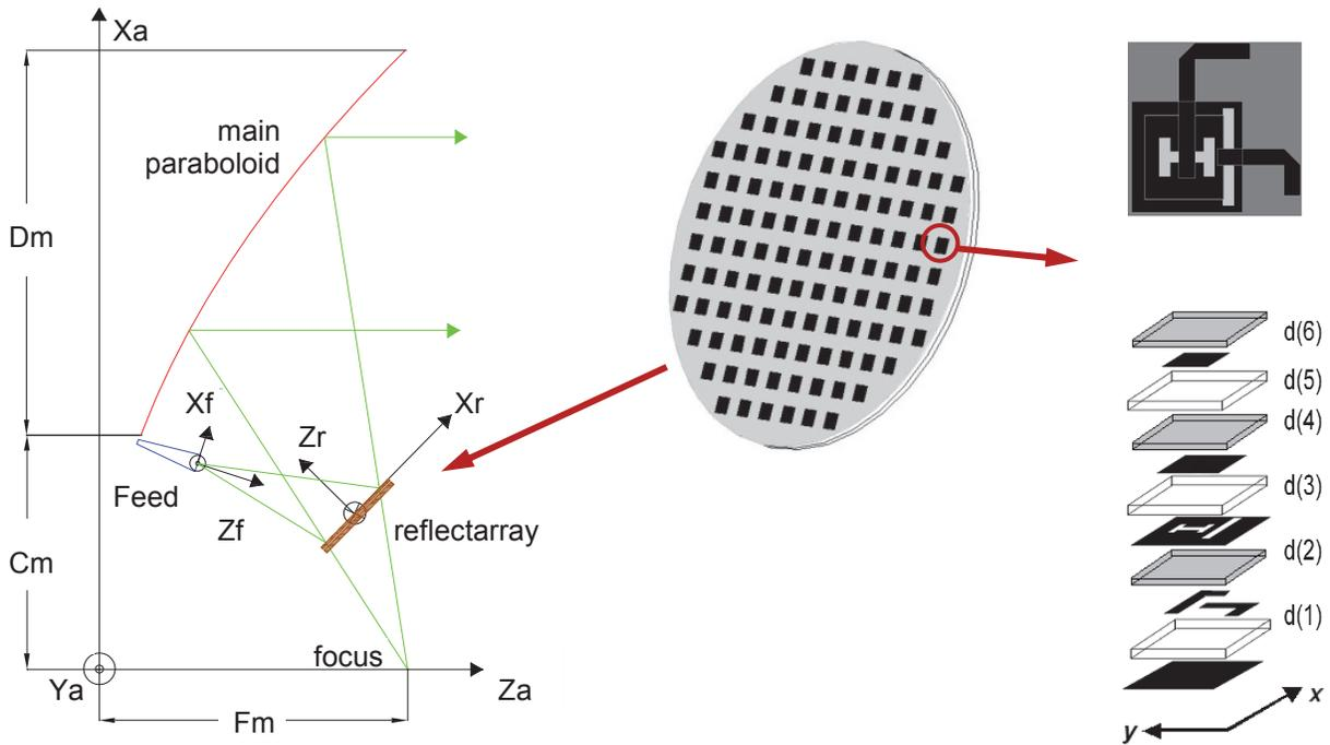
Fig. 1. Scheme of the dual-reflector configuration.
