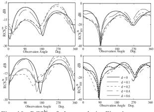
Fig. 10. RCS<sup>bi</sup> of the crack in Fig. 1 versus observation angles  $\phi_{o}$  for different dielectric thicknesses where  $a = 0.2\lambda$ ,  $b = 1\lambda$ ,  $c = 0.25\lambda$ ,  $h = 0.1\lambda$ ,  $\varepsilon_2 = 2.5 - j0.05$  and  $\varepsilon_3 = 1$  at  $\phi_i = 45^{\circ}$  and  $\theta_i = 30^{\circ}$ .
