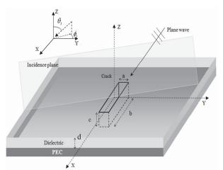
Fig. 1. Geometry of a narrow 3D-dimensional rectangular crack in an infinite ground plane underneath a dielectric layer.
