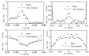
Fig. 5. Comparison between magnetic current of DIES and FEM for the crack of Fig. 1 with  $a = 0.1\lambda$ ,  $b = 0.8\lambda$ ,  $c = 0.25\lambda$ ,  $h = 0.1\lambda$ ,  $\varepsilon_2 = 3.2 - 0.1j$ ,  $\varepsilon_3 = 1$  for horizontal polarizations (H-Polarization) when  $\phi_i = 0^\circ$  and  $\theta_i = 45^\circ$ .
