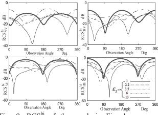
Fig. 9. RCS<sup>bi</sup> of the crack in Fig. 1 versus observation angles  $\phi_0$  or materials of table 1 where  $a=0.2\lambda$ ,  $b=1\lambda$ ,  $c=0.25\lambda$ ,  $h=0.1\lambda$  and  $\varepsilon_3=1$  at  $\phi_i=30^\circ$  and  $\theta_i=30^\circ$ .
