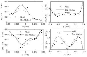
Fig. 6. Comparison between magnetic current of DIES and MoM for the crack of Fig. 1 with:  $a = 0.1\lambda$ ,  $b = 0.8\lambda$ ,  $c = 0.25\lambda$ ,  $h = 0.1\lambda$ ,  $\varepsilon_2 = 3.2 - 0.1j$  and  $\varepsilon_3 = 1$  for vertical polarizations (E-Polarization) at  $\phi_i = 0^\circ$  and  $\theta_i = 45^\circ$ .
