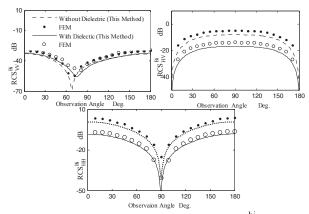
Fig. 7. Bistatic radar cross sections (RCS<sup>bi</sup>) of the crack in Fig. 1 at various observation angles  $\phi_o$  with  $a=0.1\lambda$ ,  $b=0.8\lambda$ ,  $c=0.25\lambda$ ,  $h=0.1\lambda$ ,  $\varepsilon_2 = 3.2 - 0.1j$  and  $\varepsilon_3 = 1$  at  $\phi_i = 0^o$ .
