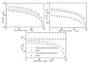
Fig. 8. RCS<sup>bi</sup> of the crack in Fig. 1 at various observation angles  $\theta_0$  with  $a = 0.1\lambda$ ,  $b = 0.8\lambda$ ,  $c = 0.25\lambda$ ,  $h = 0.1\lambda$ ,  $\varepsilon_2 = 3.2 - 0.1j$  and  $\varepsilon_3 = 1$  at  $\phi_1 = 0^\circ$  and  $\theta_1 = 45^\circ$ .
