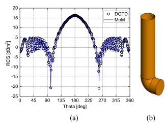
Fig. 4. (a) the bistatic RCS results and (b) the inset of the bending air-inlet model.
