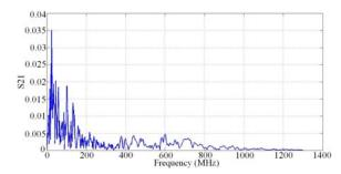
Fig. 11. Frequency magnitude response for transmission path A.
