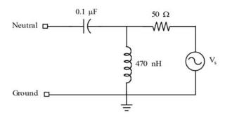
Fig. 2. High-pass filter used for isolating measurement equipment.
