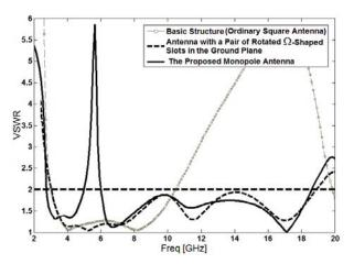
Fig. 3. Simulated VSWR characteristics for the various square monopole antenna structures shown in Fig. 2.
