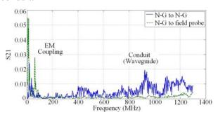
Fig. 21. Frequency response for transmission path E (wing to wing): direct and field probe.
