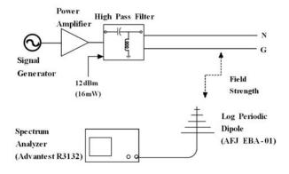
Fig. 6. Electric field measurement setup.
