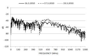
Fig. 7.  $S_{21}$  measured at 5pm on separate days for path A.
