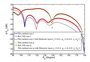
Fig. 5. Normalized RCS as a function of incident angles for case e, and with a dielectric layer of case f.
