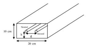
Fig. 24. Conduit cross-sectional view including neutral and ground.
