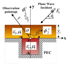
Fig. 1. Geometry of the filled rectangular crack underneath a coating layer in an infinite ground plane.
