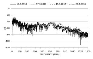
Fig. 8.  $S_{21}$  measured at 5pm on separate days for path B.
