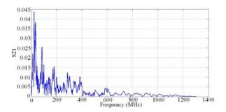
Fig. 15. Frequency magnitude response for transmission path C.
