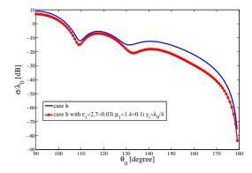
Fig. 7. Normalized backscattering RCS of the narrow crack of case h and this case with a  $\lambda_0$  / 4 dielectric layer of  $\varepsilon_1 = 2.7 + 0.03i$  and  $\mu_1 = 1.4 + 0.1i$ .
