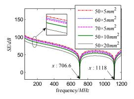
Fig. 7. Effect of aperture dimensions on SE.
