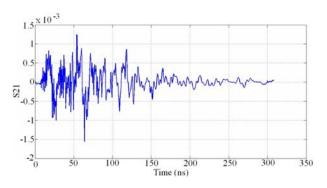
Fig. 16. Impulse response for transmission path C.
