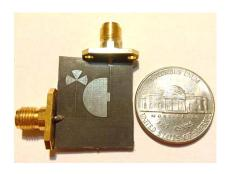
Fig. 18. The photograph of the proposed filter.
