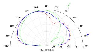
Fig. 11. Scattering far-field pattern for a crack where w = b, 2ka = 5,  $y_t = \lambda_0 / 7$ , and dielectric filled material characteristics are depicted in the figure legend
