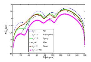
Fig. 6. Normalized bistatic RCS of the crack versus observation angle for various coated dielectric materials of case g.
