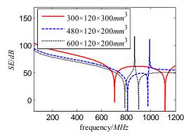
Fig. 8. Effect of enclosure dimensions on SE.
