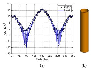
Fig. 2. (a) the bistatic RCS results and (b) the inset of the straight air-inlet model.
