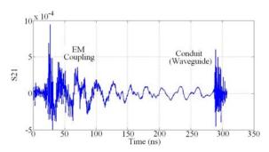
Fig. 20. Impulse response for path E (wing to wing).
