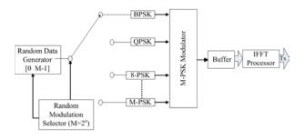
Fig. 4. UWB-OFDM signal generator with multi-modulation.
