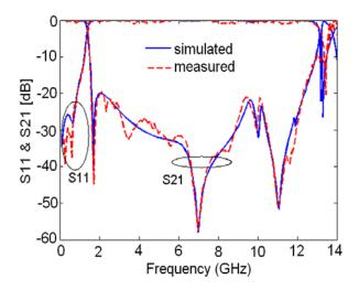
Fig. 19. The simulated and measured results of the proposed filter.
