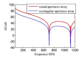
Fig. 14. Effect of aperture shape on SE.
