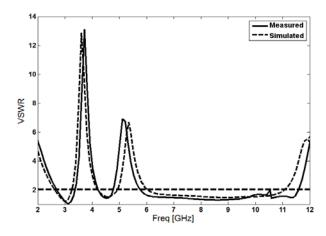
Fig. 8. Measured and simulated VSWR characteristics for the proposed antenna.
