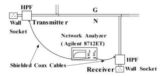
Fig. 1.  $S_{21}$  transmission measurement setup.
