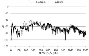
Fig. 9. S<sub>21</sub> measured at different times for path E.
