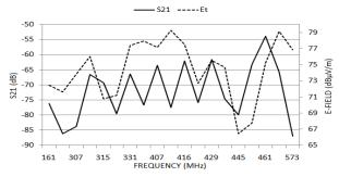
Fig. 10.  $S_{21}$  and electric field measurements (161 MHz to 572.5 MHz).
