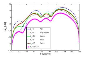
Fig. 6. Normalized bistatic RCS of the crack versus observation angle for various coated dielectric materials of case g.
