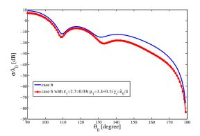
Fig. 7. Normalized backscattering RCS of the narrow crack of case h and this case with a  $\lambda_0 / 4$  dielectric layer of  $\varepsilon_1 = 2.7 + 0.03i$  and  $\mu_1 = 1.4 + 0.1i$ .
