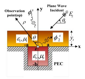
Fig. 1. Geometry of the filled rectangular crack underneath a coating layer in an infinite ground plane.
