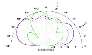
Fig. 10. Scattering far-field pattern for an empty crack where w = b and 2ka = 15.
