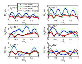
Fig. 2. Magnetic current densities on the crack (|x| < a, y = 0) computed by the proposed method and FEM for cases a and b.
