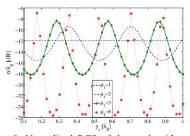
Fig. 9. Normalized RCS of the crack with  $w = 0.2\lambda_0$ ,  $b = 0.2\lambda_0$ ,  $\varepsilon_r = 2.7 + 0.03i$ ,  $\mu_r = 1$  versus paint thickness for different permeabilities.
