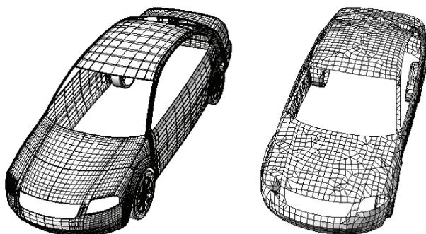
Fig. 6. Original (left) and meshed (right) vehicle.
