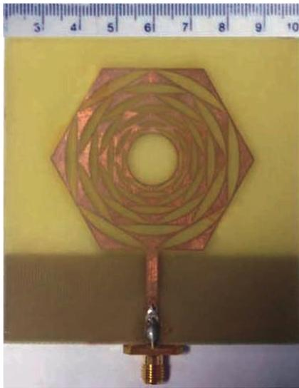
Fig. 9. Photograph of the realized Fractal antenna.
