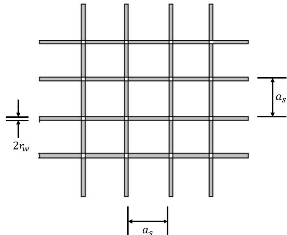
Fig. 1. Wire-mesh screen with square apertures [22].
