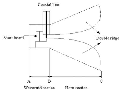
Fig. 1. Diagram of the dual-ridge horn antenna.
