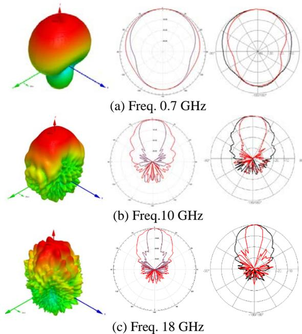
Fig. 9. Patterns: simulation (left) and measured (right).
