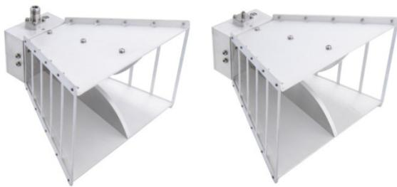
Fig. 10. Photographs of fabricated horn antenna.
