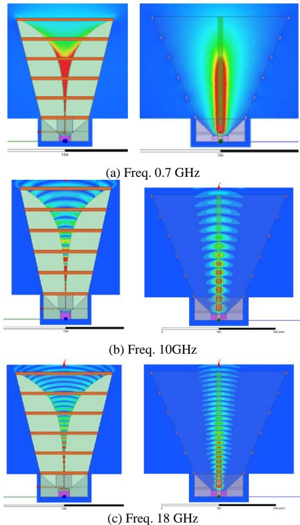
Fig. 8. E Field of designed broadband horn antenna.
