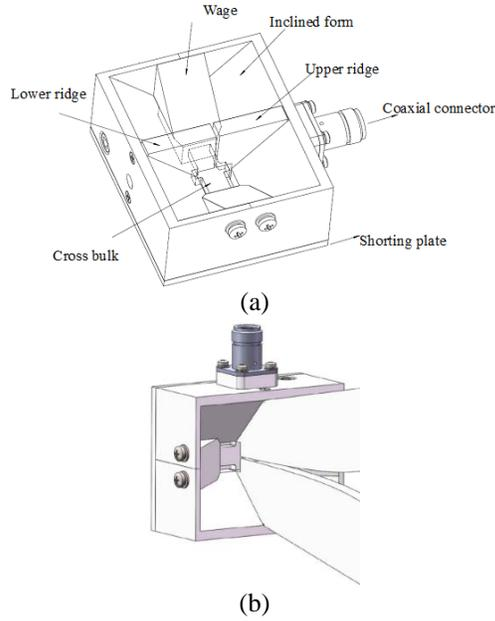
Fig. 3. Structure of rear cavity.
