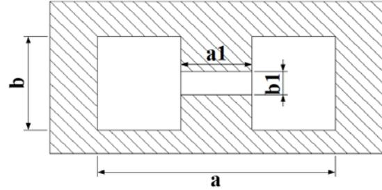
Fig. 2. Cross section of double-ridged waveguide.
