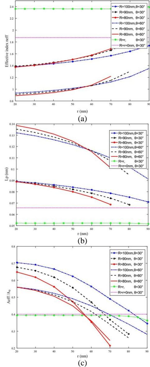
Fig. 5. Dependence of the modal properties of the fundamental hybrid mode with the different  $R$  and  $r$ ; (a) the effective refractive index ( $n_{eff}$ ), (b) the propagation length ( $L_p$ ), and (c) normalized the effective area ( $A_{eff}/A_0$ ).
