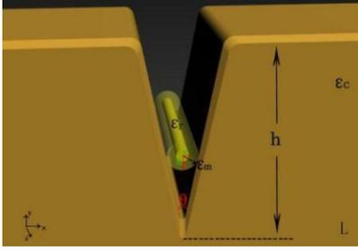
Fig. 1. Geometry of the proposed hybrid groove waveguide. The silicon slice (height  $h = 600$  nm, width  $L = 800$  nm,  $\epsilon_c = 12.25$ ) is used as the V-groove substrate with the angle ( $\theta$ ), and the silver nanowire (the radius is denoted by  $r$ ,  $\epsilon_m = -129 + 3.3i$ ) [9] is coated with low-index dielectric  $SiO_2$  (the radius is denoted by  $R$ ), thus, the thickness of the  $SiO_2$  ( $\epsilon_r = 2.25$ ) layer is denoted by  $d = R - r$ .
