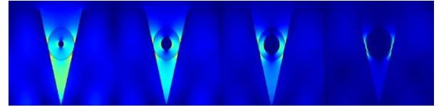
Fig. 3.  $S_z$  distributions of the fundamental mode with different  $r = 20, 40, 60, 90$  at  $\theta = 30^\circ$  and  $R = 100$  nm.
