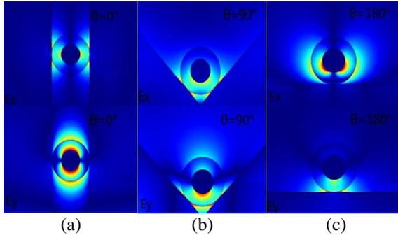
Fig. 4. Field distributions of the dominant electric component  $E_x$  and  $E_y$  on various angle.
