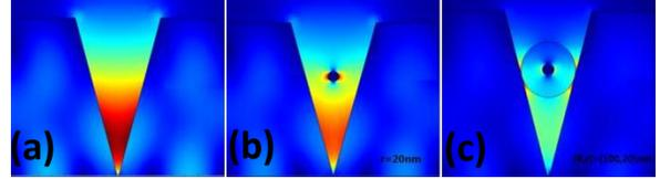
Fig. 2.  $S_z$  distributions of the fundamental mode of hybrid groove waveguide with different geometries: (a) conventional V-groove waveguide ( $\theta = 30^\circ$ ), (b) V-groove waveguide with metal nanowire ( $\theta = 30^\circ$ ,  $r = 20$  nm), and (c) the proposed hybrid V-groove waveguide ( $\theta = 30^\circ$ ,  $[R, r] = [100, 20]$  nm).
