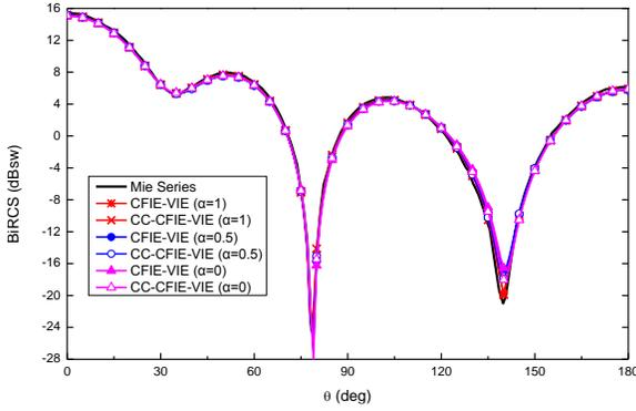
Fig. 2. Bistatic RCS for a PEC sphere of radius  $0.5\lambda$  coated with  $0.075\lambda$  thick homogeneous electrical anisotropic dielectric at  $\varphi=0^\circ$ , illuminated by a  $\theta$ -polarized plane wave with the incident angle  $\theta^i=0$ ,  $\varphi^i=0$ .
