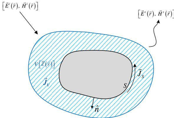
Fig. 1 Composite PEC-electrical anisotropy object under plane EM wave illumination.
