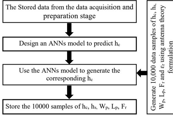
Fig. 3. Parameter substitution and optimization.
