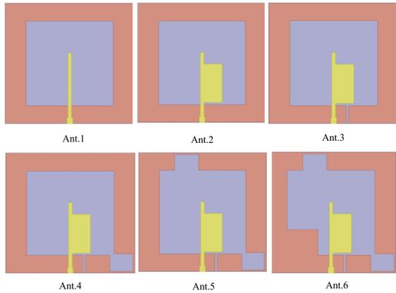
Fig. 2. Design steps of the proposed wide-slot antenna.
