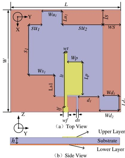
Fig. 1. Geometry of the proposed wide-slot antenna. ( $L=70$ ,  $W=65$ ,  $su_1=8.4$ ,  $Wu_1=13$ ,  $Lu_1=8.7$ ,  $su_2=25.9$ ,  $s_1=32$ ,  $Ws_1=16.6$ ,  $Ls_1=13.7$ ,  $lf=3.1$ ,  $wf=3.1$ ,  $ds=1.2$ ,  $d_1=13.35$ ,  $Wd_2=12.5$ ,  $Ld_1=9.4$ ,  $Wd_1=10.2$ ,  $Wp=9.9$ ,  $Lp=21$ ,  $lt=35$ ,  $wt=1.9$ ,  $ls=9.65$ ,  $ws=11.35$ ). (Unit: mm).
