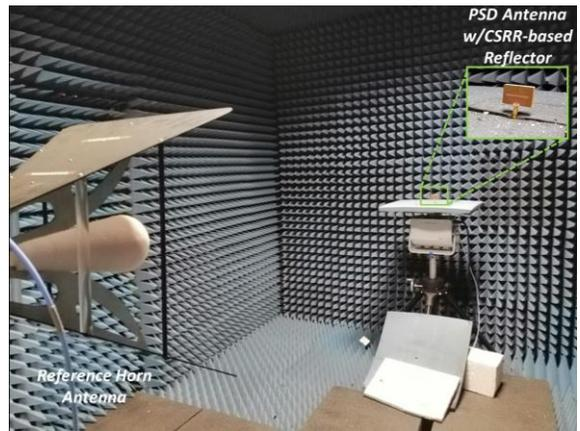
Fig. 7. The measurement setup of the proposed PSD antenna with CSRR-based reflector.
