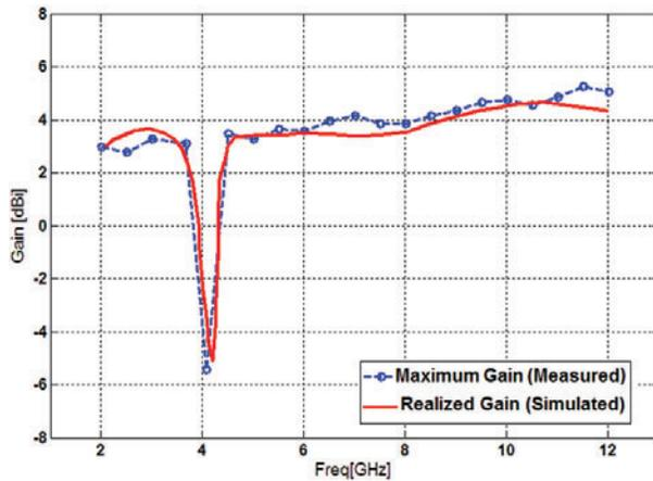
Fig. 14. Measured maximum gain for the proposed antenna.
