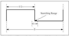
Fig. 26. Differentiation of a collision signal.
