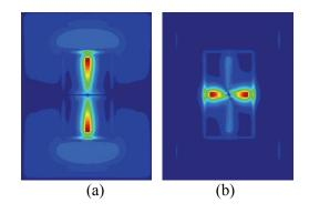
Fig. 5. FDTD simulation of E-field patterns: (a) the longest dipole is excited by a plane wave at  $f_0$  having the E-field parallel to the dipole itself; (b) the diode quad generates a  $2f_0$  frequency component which is emitted by the shortest dipole.
