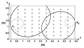
Fig. 6. Planning result on the vertical section (B) of Fig. 5. Crosses represent  $\{\underline{r}_T\}$  (read test points). R<sub>1</sub> and R<sub>2</sub> reader's antenna locations. Continuous line ellipses show the uniform covered zone of readers. Dotted line ellipses show the zone where the field exceeds the regional safety regulations.
