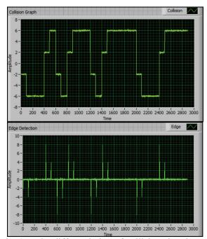
Fig. 25. The differentiation of collision signal.
