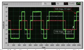
Fig. 22. Ending location of preambles in collision.
