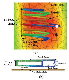
Fig. 9. (a) Perspective view and (b) crosssectional view of the experimental NMHA structure.
