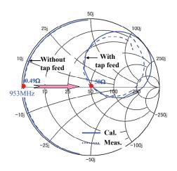
Fig. 11. Input impedances with and without tap feed.
