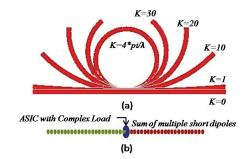
Fig. 9.Test setup of the curvature of a center-fed dipole: (a) showing the variation of curvature (K); (b) the tag composed of a summation of cylindrical parts and a complex load.
