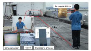
Fig. 19. Read range measurement.
