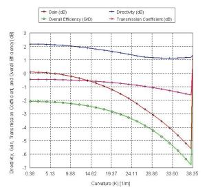
Fig. 13. Effect of curvature (K) on the directivity, gain, overall efficiency, and transmission coefficient of a center-fed dipole tag at 915 MHz.
