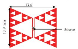
Fig. 11. Antenna structure (multiple Sierpenski antennas).
