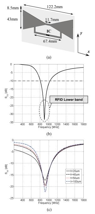
Fig. 3. (a) T-match folded bow-tie RFID antenna, (b) Return loss of the antenna with radiation element made of copper. (c) Return loss with radiation element made of SWCNT.
