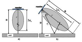
Fig. 3. Ellipsoid model of radiation pattern of readers antenna in front of a wall, a) orthogonal incidence, b) oblique incidence.
