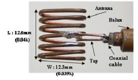
Fig. 10. Photograph of the fabricated antenna.
