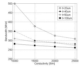
Fig. 4. The bandwidth of SWCNT antenna versus conductivity (f = 921 MHz).
