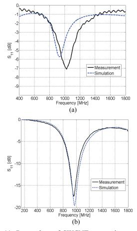
Fig. 11. Return loss of SWCNT composite antenna, (a) T-match bow-tie, and (b) MLA.
