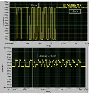
Fig. 12. Acquired collision signal.
