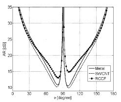
Fig. 7. *E*-plane axial ratio of bow-tie antenna with different radiating element.
