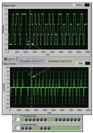
Fig. 28. Collision signal and differentiation.
