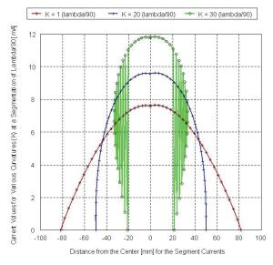
Fig. 20. Effect of the tag curvature on the segment currents for damp meshing guidelines (dense segmentation process).
