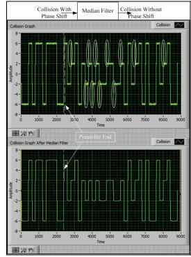
Fig. 37. The effect of median filter.
