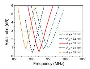
Fig. 7. Simulated axial ratio versus frequency for different inner radii  $(R_2)$ .
