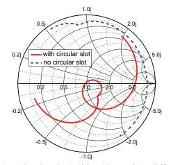
Fig. 3. Simulated Smith Chart for different circular slot radii  $(R_3)$ .
