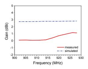
Fig. 12. Measured and simulated antenna gains versus frequency for the proposed antenna.
