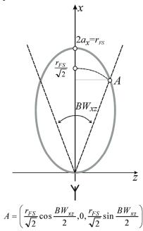
Fig. 2. Geometrical construction for the determination of the axes of the ellipsoid approximating the free-space read zone.
