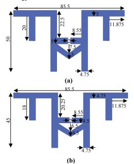
Fig. 2. The final designs for (a) 866MHz and (b) 915MHz, respectively all dimensions are in (mm).
