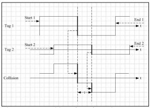
Fig. 17. Superposition of two formation-0 symbols.
