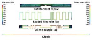
Fig. 4. Current distribution of commercial RFID tags as compared to the typical dipole antenna.
