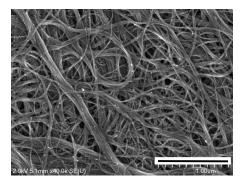
Fig. 2. SEM micrograph of bucky-paper made of SWCNTs (scale bar 1  $\mu$ m).
