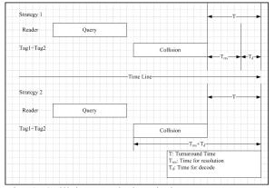
Fig. 4. Collision resolution timing strategy.
