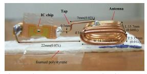
Fig. 18. The RFID tag structure using the NMHA.
