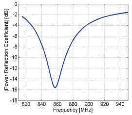
Fig. 3. The input impedance and power reflection coefficient for design 1 shown in Fig. 2(a).
