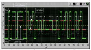
Fig. 32. Superposition of tag responses without phase shift.
