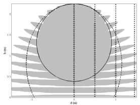
Fig. 4. Interrogation region prediction in case of the reader's antenna pointing toward the ground. Comparison between free-space model (continuous line ellipse), two-rays model (dotted line ellipse), full ray-tracing (grey region) and measurements shown by means of circle and cross markers. Circles concern reading locations, crosses non-reading locations. Reader power: 1.2 W EIRP.
