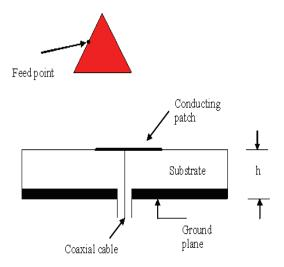
Fig. 1. Antenna structure (triangular patch).
