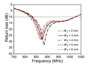
Fig. 6. Simulated return loss for different widths of meandered slot section  $(W_1)$ .
