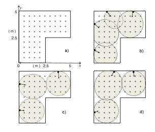
Fig. 8. L-shaped environment wherein network coverage is planned with different constraints. a) set-up with  $\{\underline{r}_T\}$  shown by stars; b) EIRP and antennas orientation (indicated by arrows) optimized; c) number of readers, EIRP and orientation optimized; d) complete optimization. Arrows show antennas' orientation, ellipses interrogation region.
