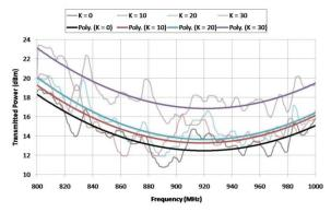
Fig. 18. Experimental analysis and polynomial curve fitting of the results for curvatures of the Alien Squiggle tag from 800-1000 MHz.
