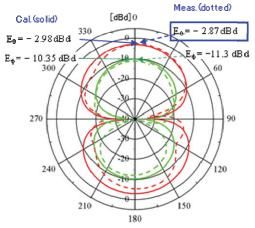
Fig. 13. Radiation patterns without metal plate.
