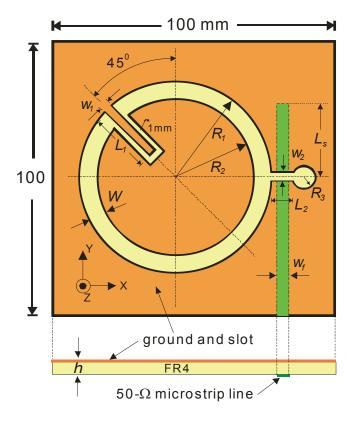
Fig. 1. Geometry of the single-layer circularly polarized annular-ring slot antenna.
