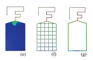
Fig. 3. Topology of inkjet-printed antenna designs of a commercial tag at US RFID band.
