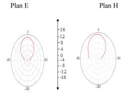
Fig. 13. Radiation pattern (Etotal) of multiple Sierpenski patch.
