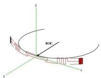
Fig. 15. Curvature setup of the Alien Squiggle tag for a given radius of curvature (ROC).
