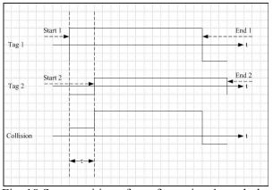
Fig. 18.Superposition of two formation-1 symbols.
