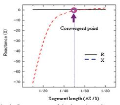
Fig. 3. Convergence of the input impedance.
