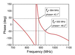
Fig. 9. Simulated phase diagram versus frequency for the proposed antenna.
