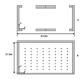
Fig. 5. Horizontal (A) and vertical (B) section of the hall used for experiment. Crosses indicate the read test points  $\{\underline{r}_T\}$ .
