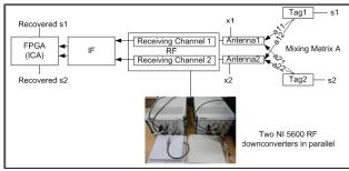
Fig. 45. ICA for two-tag collision resolution experiment configuration.
