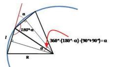
Fig. 8. Relationship between tag effective length  $(L_e)$  and differential deployment angle  $(\alpha)$ .
