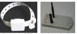
Fig. 9. Active RFID wristband tag and reader.
