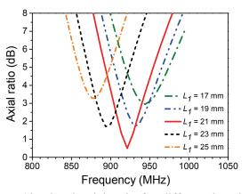
Fig. 5. Simulated axial ratio for different lengths of meandered slot section  $(L_1)$ .
