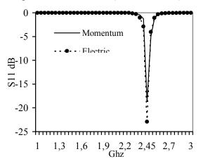
Fig. 7. Return loss of both physical and model patch (second structure).
