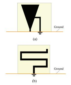
Fig. 10. Monopole configuration of SWCNT composite antennas, (a) T-match bow-tie, and (b) MLA.
