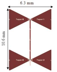
Fig. 6. Antenna structure (second structure).
