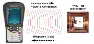
Fig. 2. A typical RFID system with handheld reader.
