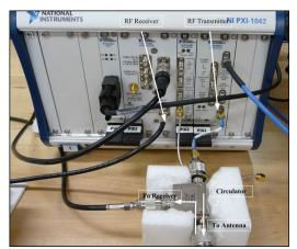
Fig. 14. RF front end connection with circulator.
