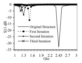
Fig. 9. Return loss of Sierpenski antenna.
