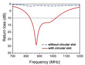
Fig. 4. Simulated return loss for different circular slot radii  $(R_3)$ .
