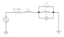
Fig. 2. Electrical model with C=0.168 nF, L= 25.11 pH, R= 66.66 Ohm,  $X_L = 1nH$  (triangular patch).
