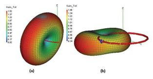
Fig. 10. 3D pattern of the tag gain: (a) during curvature values of  $K < 4\pi/\lambda$ ; (b) at  $K = 4\pi/\lambda$ .
