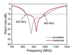
Fig. 8. Measured and simulated return loss of the proposed antenna.
