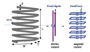
(a) Perspective view (b) Electrical equivalent configuration
