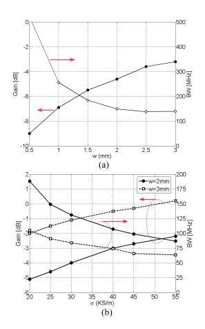
Fig. 9. Gain-bandwidth diagram of SWCNT MLA versus (a) w ( $\sigma$  = 25KS/m, t = 50 $\mu$ m, f = 950.4 MHz), (b)  $\sigma$  (t = 100 $\mu$ m, f = 976.35 MHz).
