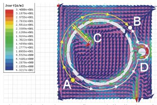
Fig. 2. Simulated current flow and distribution of the proposed antenna at 915 MHz.
