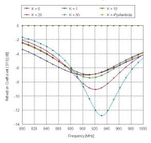
Fig. 11. Effect of curvature (**K**) at different frequencies.
