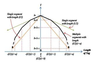
Fig. 7. Current distribution of tag antenna depending on the number of segments and length.
