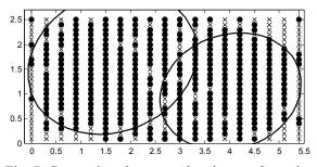
Fig. 7. Comparison between planning results and measurements. Ellipses show the planned uniform read zone as estimated by the electromagnetic two-rays tool. Crosses and dots show measured non reading and reading points, respectively.
