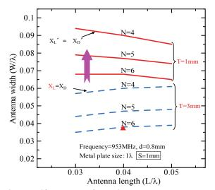
Fig. 5. Self-resonance for various T.
