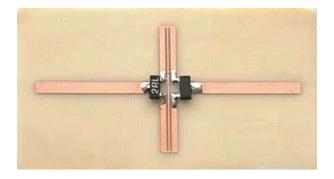
Fig. 4. Photograph of the proposed frequency doubling tag. The length of the longest  $l_0$  dipole, corresponding to the double of the shortest one  $l_1$ , is  $l_0 = 2l_1 = 32$ mm. The substrate thickness is h = 0.8mm while its dielectric constant is  $\varepsilon_r = 3.38$ .
