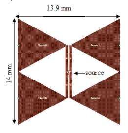
Fig. 4. Antenna structure (first structure).
