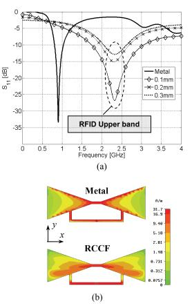
Fig. 5. (a) Return loss of RCCF antenna, (b) Current distribution on the radiation element at resonant frequency (f = 2330 MHz).
