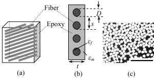
Fig. 1. (a) RCCF composite, (b) Cross-view, (c) Optical micrograph of RCCF Composite (scale bar 50  $\mu$ m).
