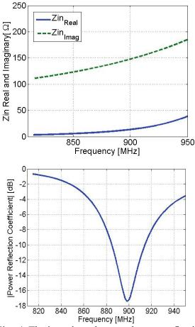
Fig. 4. The input impedance and power reflection coefficient for design 2 shown in Fig.2 (b).
