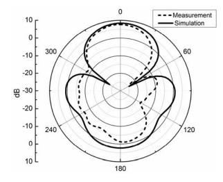
Fig. 4. Simulated and measured H-plane of the proposed antenna at 5.8 GHz.
