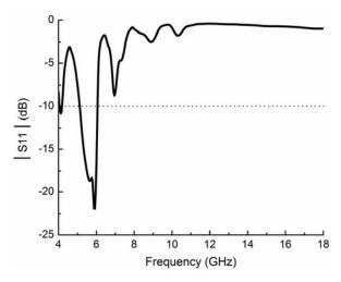
Fig. 7. Simulated reflection coefficient magnitude of the antenna array.
