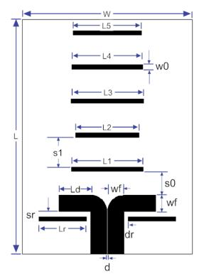
Fig. 1. Schematic diagram of the proposed quasi-Yagi antenna.
