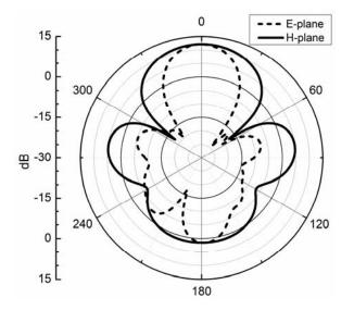
Fig. 8. Simulated E- and H-planes of the antenna array at 5.8 GHz.
