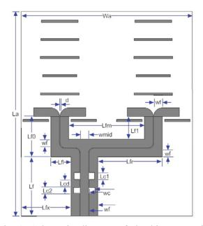
Fig. 6. Schematic diagram of the binary quasi-Yagi antenna array.
