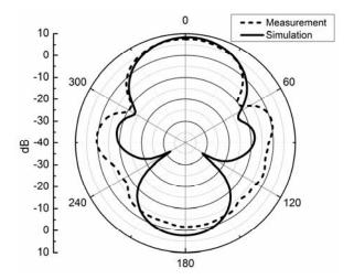
Fig. 3. Simulated and measured E-plane of the proposed antenna at 5.8 GHz.
