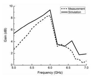
Fig. 5. Simulated and measured peak gain variation against frequency for the proposed antenna.
