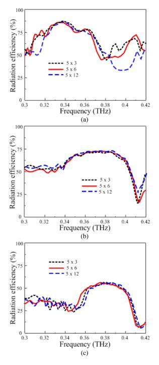
Fig. 2. Antenna gain with different numbers of patch cells and different substrate thicknesses: (a)  $H = 80 \mu m$ , (b)  $H = 40 \mu m$ , and (c)  $H = 20 \mu m$ .
