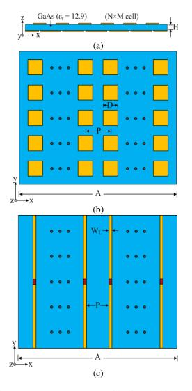
Fig. 1. Antenna geometry: (a) side view, (b) front view of top surface, and (c) front view of bottom surface.
