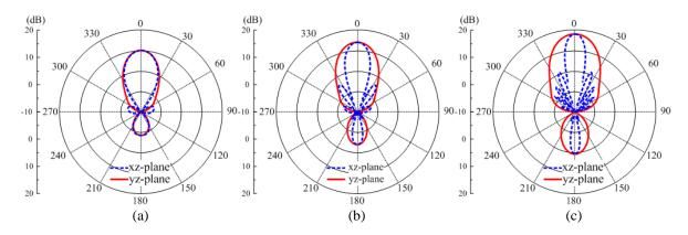
Fig. 5. Antenna radiation patterns for different numbers of patch cells at  $H = 40 \ \mu\text{m}$ : (a) 5×3, (b) 5×6, and (c) 5×12.
