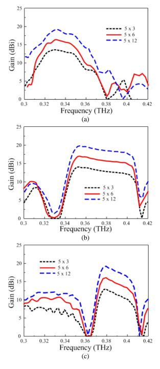
even though the leaky-wave slit is open to free space. However, the gain value associated with both back radiations increased with an increase in the number of patch cells. Interestingly, the back radiation decreased when the substrate thickness increased.
