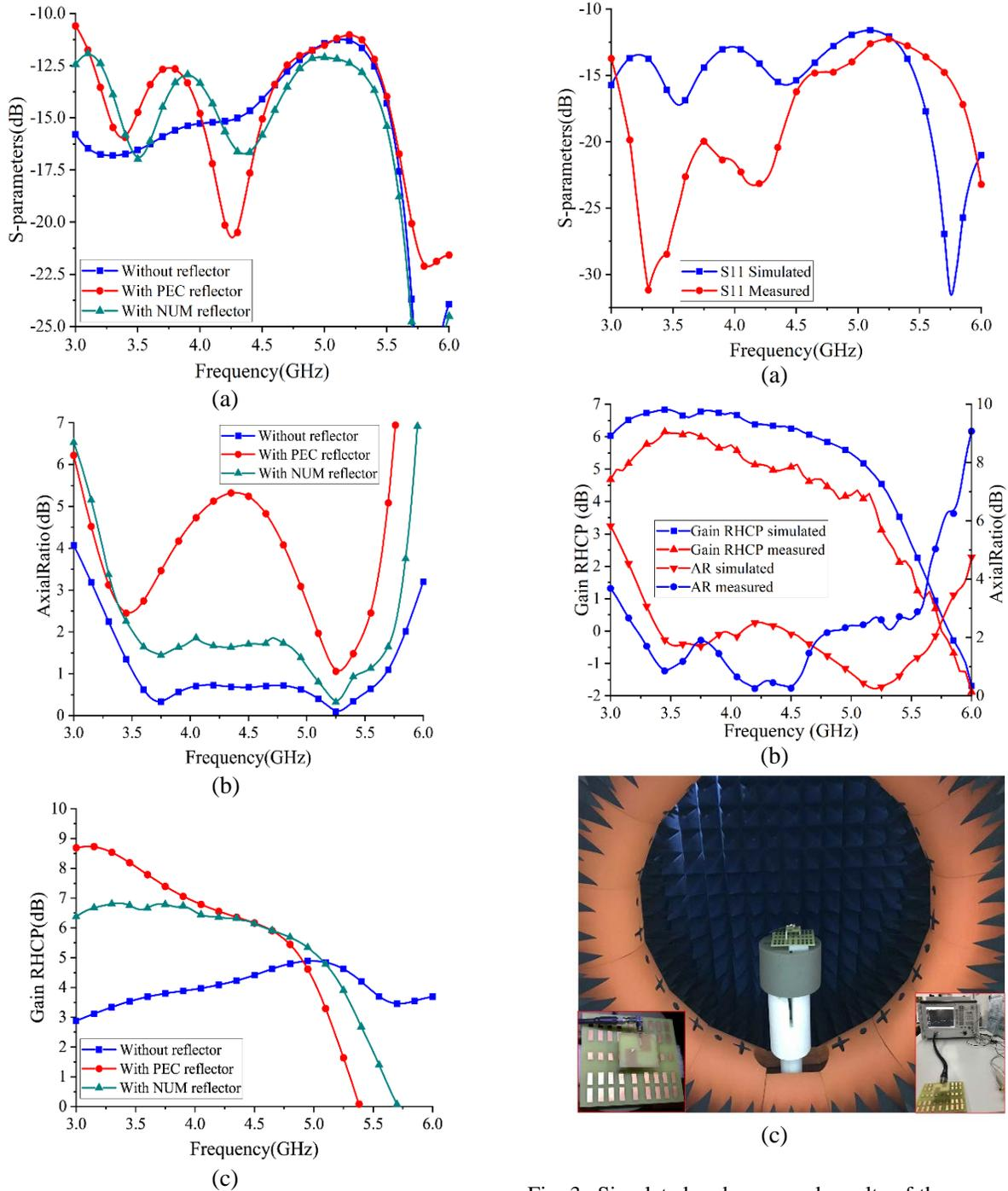
Fig. 2. Comparisons of different antennas' performances. (a) S<sub>11</sub> of the antenna. (b) AR of the antenna. (c) Gain of the antenna.
