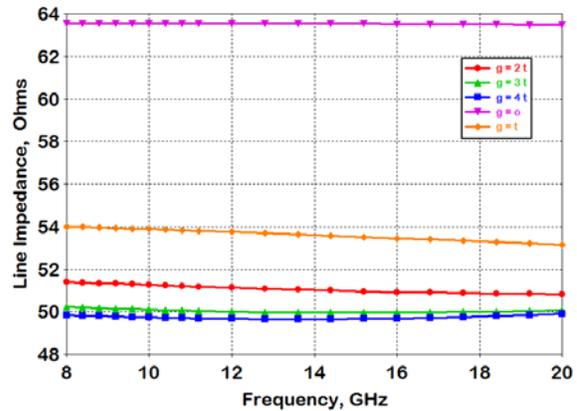
Fig. 3. Effect of the PMC lid on the characteristic impedance of the microstrip line,  $g = h-t$ .
