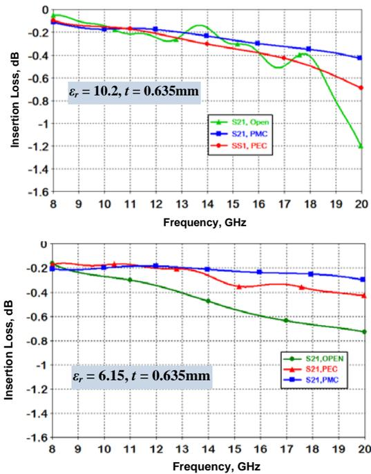
Fig. 2. Insertion losses of a straight microstrip line for different packaging cases, and for two different relative permittivities.
