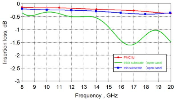
Fig. 4(b). Comparison between bended microstrip line on thin or thick substrates, open and with PMC lid 3t above substrate.
