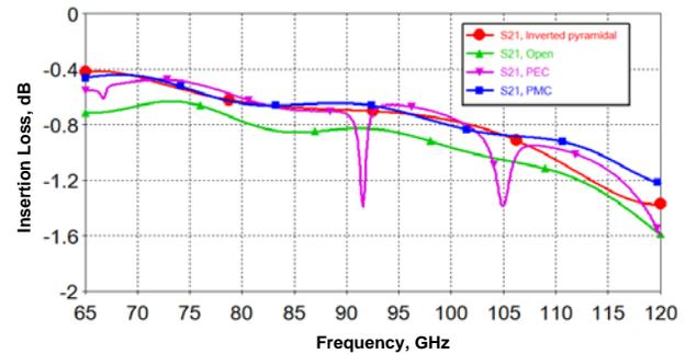
Fig. 6(c).  $S_{21}$  of the right angle microstrip line for the open case, PEC lid, PMC lid, and inverted pyramidal-shaped pin lid.
