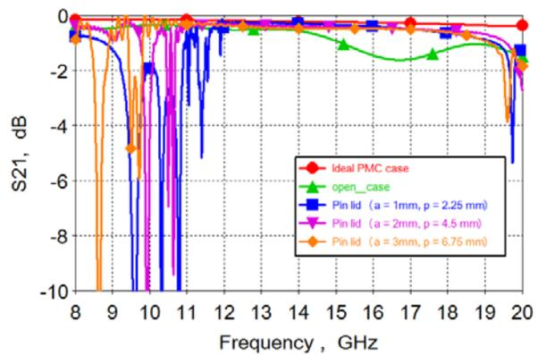
Fig. 5 (c). Simulated  $S_{21}$  of the right angle microstrip line with different  $a$  and the same  $a/p$ .
