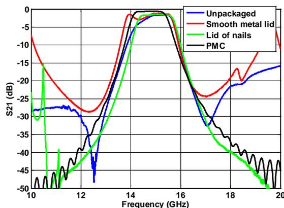
Fig. 7(b). The microstrip filter measurement response in three cases compared with the simulated PMC packaging case.
