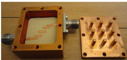
Fig. 7(a). Photo of the microstrip coupled line filter with the pin lid cover on the side.
