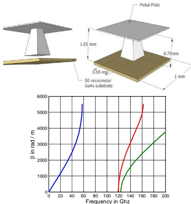
Fig. 6(b). Dispersion diagram obtained from the for one cell with inverted pyramidal-shaped pins that provide the wider bandwidth than the rectangular pins.
