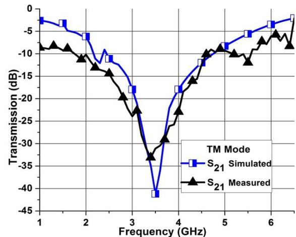
Fig. 12. Measured and simulated transmission for TM mode.
