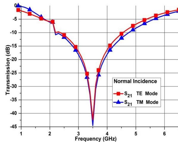
Fig. 2. Transmission behaviour of the FSS at normal incidence.
