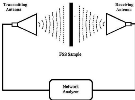
Fig. 9. FSS free-space measurement method.
