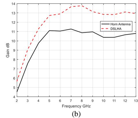
Fig. 4. Simulated (a)  $S_{11}$  and (b) gain
