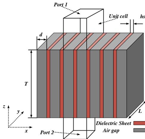
Fig. 2. Proposed DS model for DSLHA module design.
