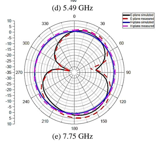
Fig. 12. E plane and H plane pattern (measured and simulated comparison).
