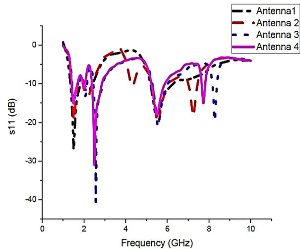
Fig. 6. S<sub>11</sub> characteristics - various stages of proposed antenna.
