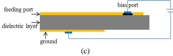
Fig. 1. Geometry of presented frequency tunable antenna: (a) the front geometry of antenna; (b) the back geometry antenna; (c) the DC voltage connection method on the FLG. ( $L_1=25$ ,  $L_g=13$ ,  $L_2=11$ ,  $L_g1=4.5$ ,  $L_3=1.5$ ,  $W_1=20$ ,  $L_4=0.7$ ,  $W_2=12$ ,  $L_5=4.5$ ,  $W_3=1$ ,  $L_6=0.6$ ,  $W_f=4.8$ ,  $L_f=13$ ,  $W_{g1}=3.5$ ) (unit: millimeter).
