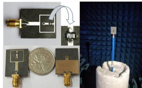
Fig. 4. The prototype of the proposed antenna.
