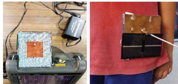
Fig. 10. Proposed wearable antenna measurement setup.
