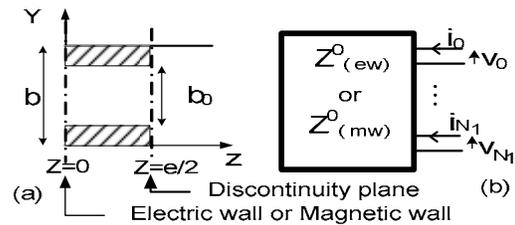
Fig. 5. (a) Side-view of half of the unit-cell for magnetic and electric wall configurations. (b) Surface impedance multiport for modeling the unit-cell.  $N_1$  denotes the number of active modes at the smallest scale.
