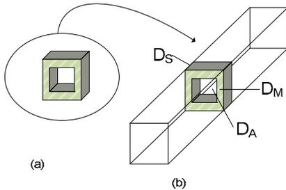
Fig. 4. (a) Initial lossless metallic pattern with a passive sub-domain  $D_S$  presenting many fine geometrical details; (b) artificial rectangular waveguide of cross section  $D_S$  in which the set of propagating and evanescent modes constitutes the basis for the electromagnetic field.
