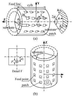
Fig. 7. Geometry of the cylindrical microstrip antenna array, frequency is at 16.2 GHz; a=76mm, h=0.254 mm, b=a+h, S=15 mm, 2L=7.2 mm,  $2b\phi_0 = 5$  mm, cylh=66 mm,  $2\phi_c = 46^\circ$ , dz=1 mm, p=0.2 mm. (a) Microstrip-line fed, (b) probe fed.
