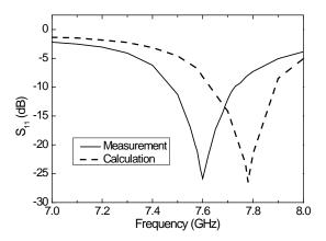
Fig. 5.  $S_{11}$  (dB) results comparison.
