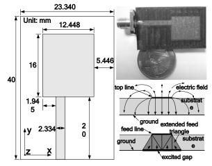
Fig. 4. Microstrip patch antenna model.
