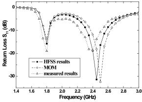
Fig. 3. Compared results of  $S_{11}$  (dB).
