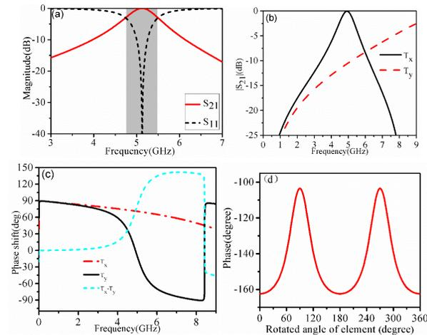
Fig. 3. (a) The scattering parameter of the element, (b) insertion loss of the element in the direction of the orthogonal polarization, (c) the transmission phase and phase difference of the element in the orthogonal direction, and (d) relationship between element rotation angle and the change of phase.
