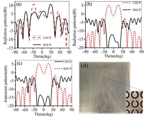
Fig. 6. (a) The simulated radiation pattern of the transmit-array under the LP horn, (b) the simulated radiation pattern of the transmit-array under the RHCP horn, (c) the simulated radiation pattern of the transmit-array under the LHCP horn, and (d) the physical samples of the transmit-array.
