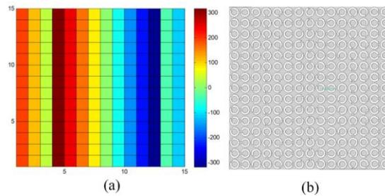
Fig. 4. (a) Rotated angle of each element and (b) Schematic diagram of transmit-array.
