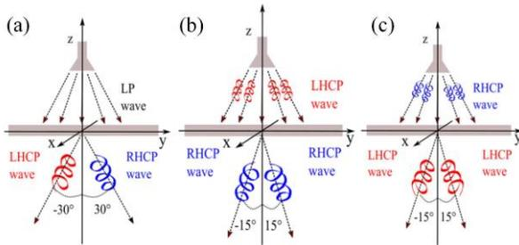
Fig. 5. Operating mode under the: (a) LP, (b) LHCP, and (c) RHCP horn antenna.
