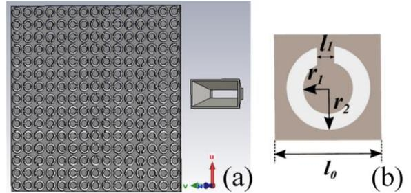
Fig. 2 (a) Conceptual model diagram of transmit-array and (b) the details of ring groove with a single split. (structure parameters:  $l_0=15$  mm,  $r_2=6$ mm,  $r_1=4$ mm, and  $l_1=2$ mm).
