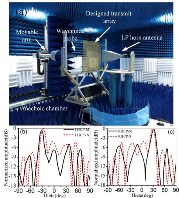
Fig. 7. (a) Overall view in an anechoic chamber, (b) measured and simulated radiation pattern of LHCP, and (c) measured and simulated radiation pattern of RHCP.
