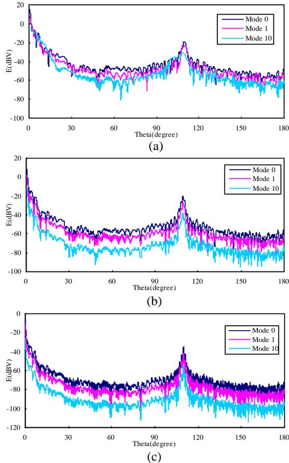
Fig. 15. The bistatic scattered field in the far field of the plane model; (a), (b) and (c) are corresponding to the operating range of 10m, 100m and 1000m respectively.
