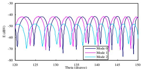
Fig. 13. The bistatic scattered field in the far field ( $\Phi=0^\circ$ ) for different mode numbers.
