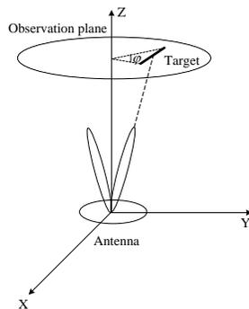
Fig. 16. The positional relationship between the antenna and the target in the far field.
