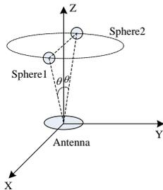
Fig. 8. Two metal spheres placed on a circle surrounding the Z-axis with an azimuthal difference of  $180^\circ$ . (The solving frequency is 30GHz, the height of the spheres is  $300\lambda$  and their radius is  $2.5\lambda$ , they are aligned with a pitch angle of  $5^\circ$  in the XOZ plane; the aperture of the parabolic antenna is  $10\lambda$  and the focus length is  $15\lambda$ .)
