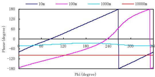
Fig. 6. The phase variation along the fix-sized circles which are placed around the propagation axis.
