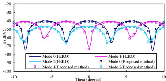
Fig. 11. The monostatic scattered field in the far field ( $\Phi=0^\circ$ ) for different mode numbers.
