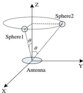
Fig. 12. Two metal spheres are placed on a circle surrounding the Z-axis with an azimuthal difference of  $90^\circ$ . (Other parameters are same with those in Fig. 8).
