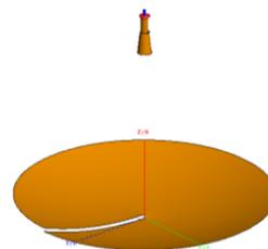
Fig. 1. The model of the spiral parabolic antenna used in numerical simulations. (The horn can be replaced by the ideal Gaussian feed source).
