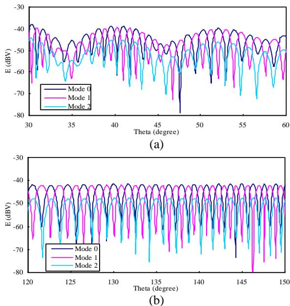
Fig. 10. The bistatic scattered field in the far field ( $\Phi=0^\circ$ ) for different mode numbers. (a) The observed pitch angle is from  $30^\circ$  to  $60^\circ$ . (b) The observed pitch angle is from  $120^\circ$  to  $150^\circ$ .
