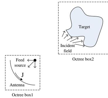
Fig. 7. The illustration of the modified octree grouping scheme for solving the electromagnetic scattering of the electromagnetic vortex generated by practical antennas.
