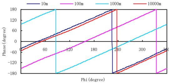
Fig. 5. The phase variation along the dynamic-sized circles which are placed along the direction of the maximum radiation.
