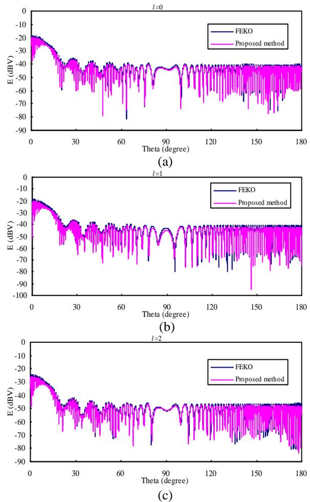
Fig. 9. The scattered electric field intensity in the far field ( $\Phi=0^\circ$ ) for the proposed method and the original method: (a)  $l=0$ , (b)  $l=1$ , and (c)  $l=2$ .
