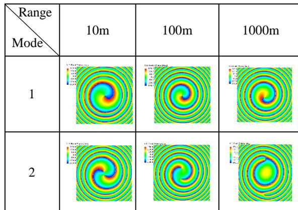
Fig. 2. The phase distribution of the electromagnetic vortex on an observation plane in different propagation distances. (The size of observation plane is 3m\*3m, 10m\*10m, 30m\*30m from left to right; the operating frequency is 10GHz; the aperture of the parabolic antenna is 36λ, the focus length is 25λ.)
