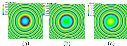
Fig. 3. The phase distribution of the mode 1 at 100km with different antenna apertures. (The aperture of the antenna is 36λ, 50λ, 80λ from (a) to (c); the size of the observation plane is 300m\*300m, other parameters are same with those in Fig. 2).
