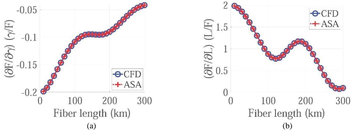
Fig. 1. Normalized ASA sensitivities of objective function (4) with respect to the fiber nonlinear coefficient  $\gamma$  and the fiber length  $L$ , for a sweep of  $L$ , as compared to the accurate but computationally expensive CFD.
