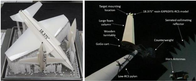
Fig. 2. Left: The additively manufactured scale models before their support structures were removed and they were sanded and metallized. Right: The measurement of the  $\sim 18.4$ -in long model in the compact chamber.
