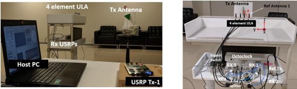
Fig. 2 Experimental setup for direction of arrival estimation.
