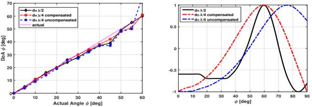
Fig. 4: DoA estimation for a four element ULA with  $d = \lambda/2$  and  $d = \lambda/4$  (with and without mutual coupling compensation). Estimated DoA vs Actual DoA for  $\theta = 90^\circ$  (left). Spatial spectrum of MUSIC algorithm for DoA detection of signal from  $\theta = 90^\circ$ ,  $\phi = 60^\circ$  (right).
