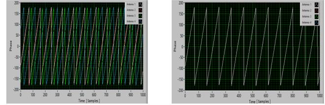
Fig. 3 Received signal. Before (left) and after (right) phase calibration.
