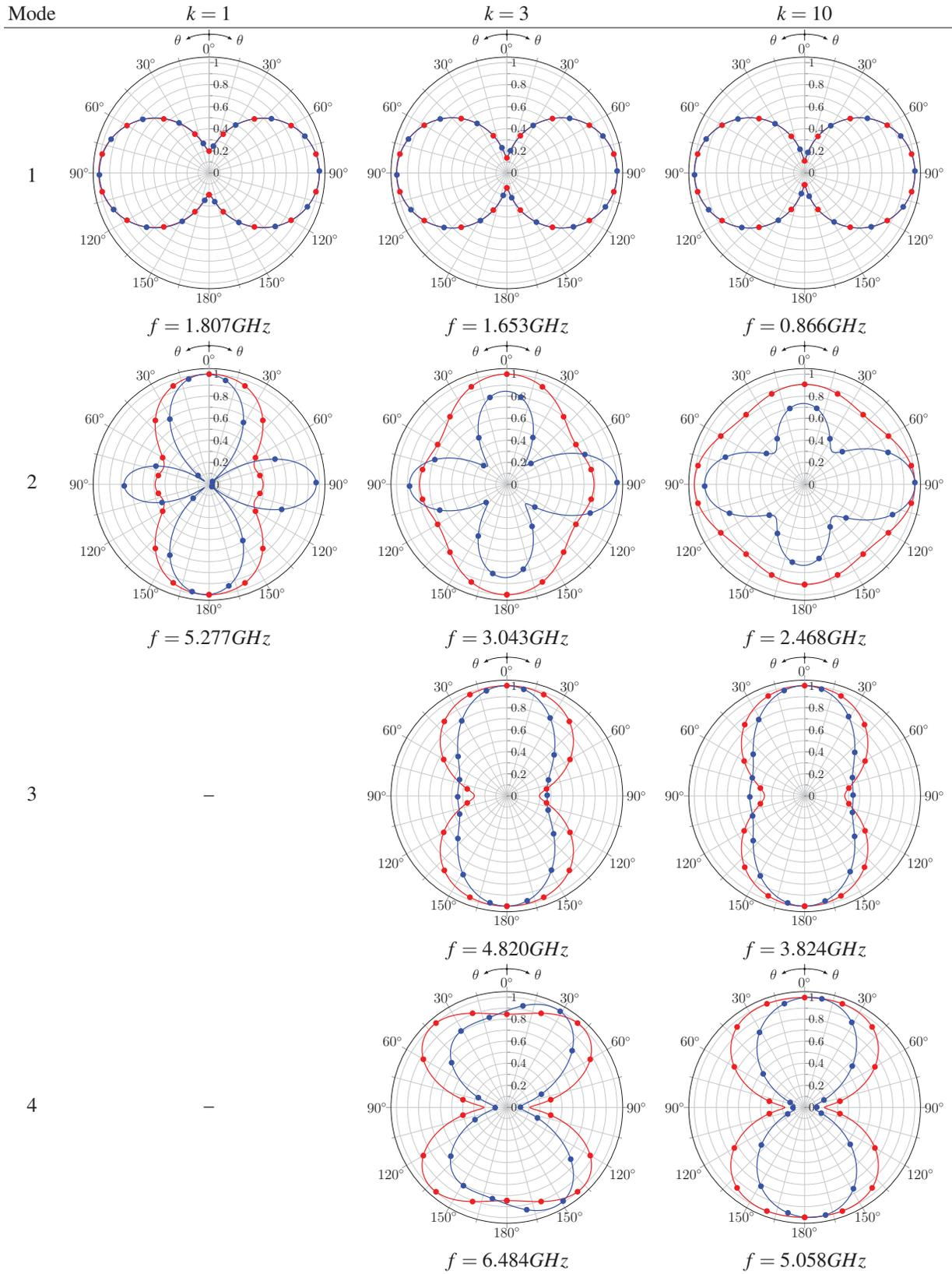
Fig. 4. The H-plane (—●—:  $\phi = 0^\circ$ ), and E-plane (—●—:  $\phi = 90^\circ$ ) normalized radiation patterns for the first four modes in frequency range  $0.8GHz \leq f \leq 8GHz$  with  $\gamma = 0.4$ .
