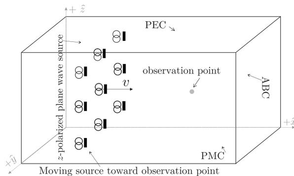
Fig. 4. Plane wave source moving toward the observer.
