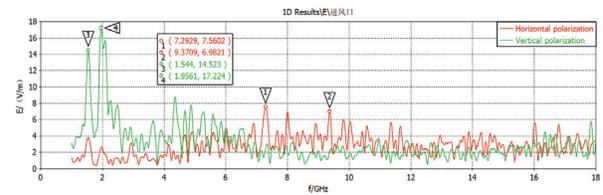
Fig. 11. Electric field intensity of the air intake.
