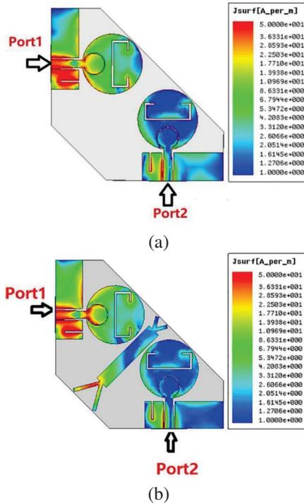
Fig. 6. Surface current distributions at 7 GHz when Port 1 acts as the exciter and Port 2 connects 50 Ω load: (a) Antenna with branch and (b) antenna without branch.
