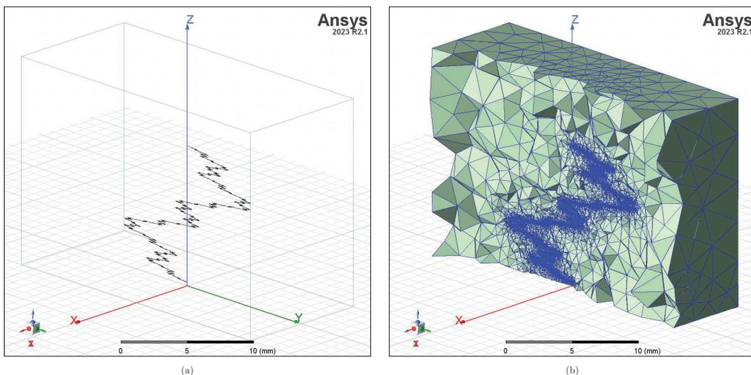
Fig. 2. HFSS 3D model for  $\gamma = 0.4$ ,  $k = 10$ . (b) Corresponding mesh.  $yz$ -plane is set to be a perfect electric symmetry boundary to for a smaller FEM model. The other outer surfaces of the mesh region is set to be radiation boundaries.
