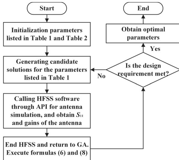
Fig. 2. Design process of the GA-generated antenna.
