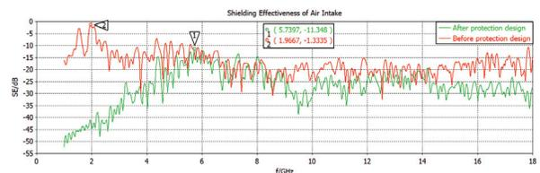
Fig. 18. Shielding effectiveness of the air intake after protection design.
