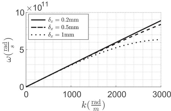
Fig. 1. Numerical dispersion for different values of  $\delta_x$ .
