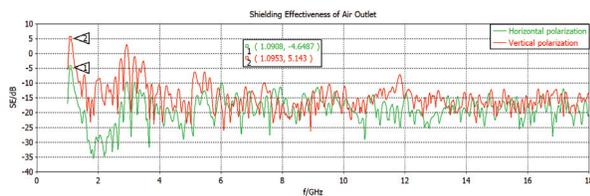
Fig. 15. Shielding effectiveness of the air outlet.
