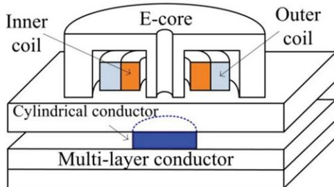
Fig. 1. E-core driver and pickup coils probe located above layered conductor containing a hidden cylindrical conductor.
