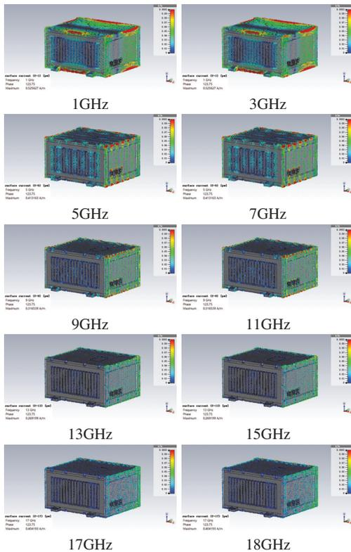
Fig. 10. Surface current distribution of the panel gaps.
