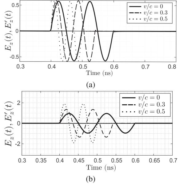
Fig. 7. Simulated signal in time domain for plane wave source moving with speed  $v$  toward observer, for different values of  $\frac{v}{c}$ : (a) Ideal plane wave source, (b) Plane wave source without resistors.
