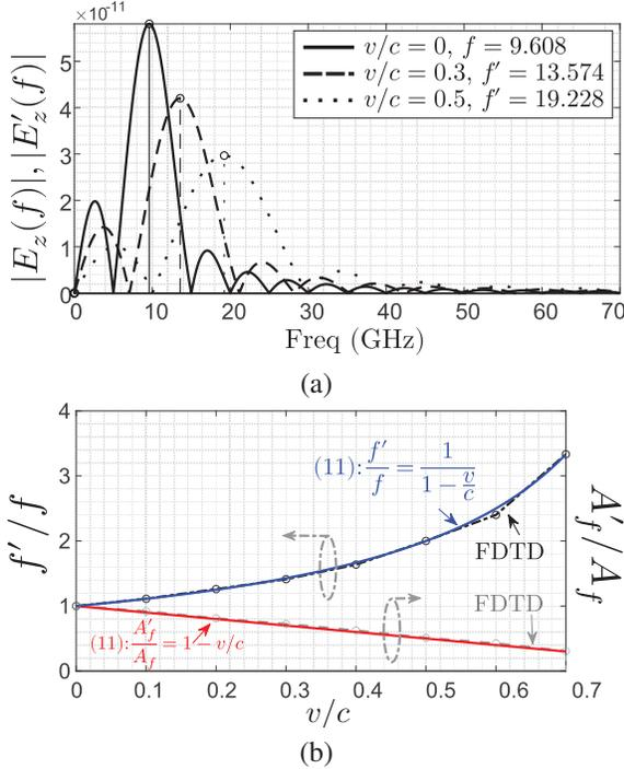
Fig. 6. Simulated results for an ideal plane wave source moving with speed  $v$  toward the observer: (a) Observed signal in the frequency domain for different values of  $\frac{v}{c}$ , (b) Doppler frequency shift and amplitude variation of the observed electric field in frequency domain versus  $\frac{v}{c}$ .
