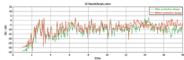
Fig. 24. Shielding effectiveness at the probe position.
