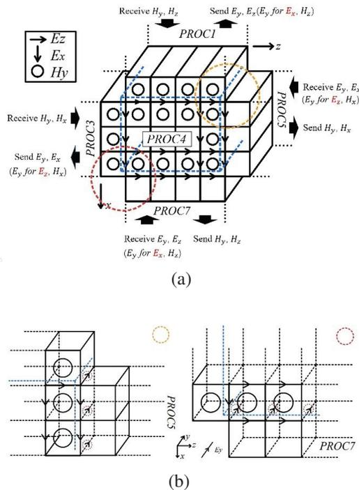
Fig. 5. The communications between PROC4 and its neighboring processes using the parallel HIE-FDTD method: (a) Overall view and (b) the communication of  $E_y$  component in the  $x$ - and  $z$ -directions.
