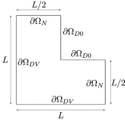
Fig. 4. Graphical description of the 2D test case.  $\partial\Omega_N$  is the section of boundary where Neumann conditions hold,  $\partial\Omega_{D0}$  and  $\partial\Omega_{DV}$  the sections where vanishing and non-vanishing Dirichlet conditions hold, respectively.
