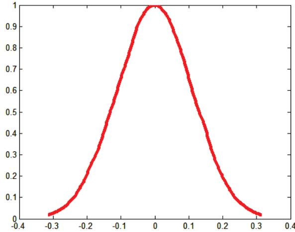
Fig. 2. Amplitude distribution of one-dimensional conical incident waves.
