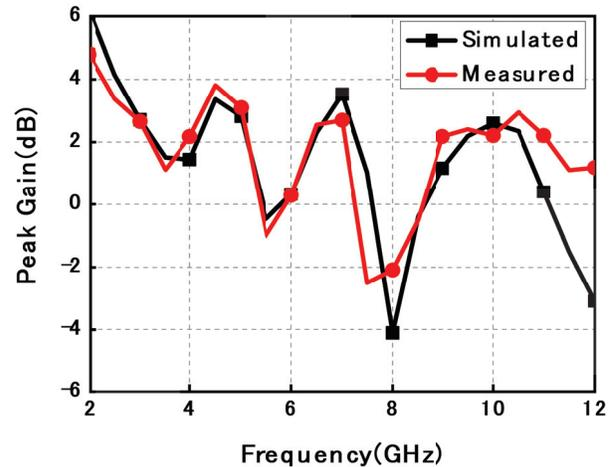
Fig. 14. Simulated and measured gain of MIMO antenna.
