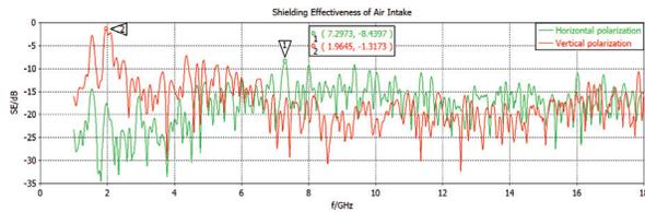
Fig. 14. Shielding effectiveness of the air intake.
