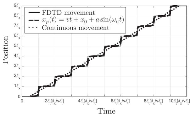
Fig. 2. Discontinuous movement of plane wave source.
