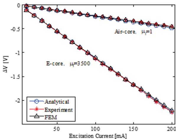
Fig. 8. The relationship between the excitation current and the change of induced voltage in the pickup coil due to the cylindrical conductor for an air-core coil ( $\mu_f = 1$ ) and an E-core coil ( $\mu_f = 3500$ ).
