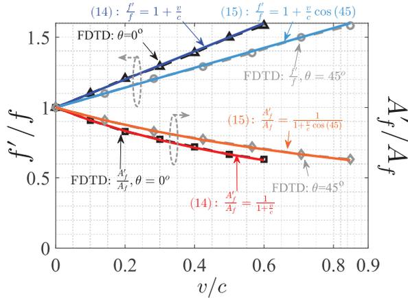
Fig. 11. Simulated Doppler frequency shift and amplitude of the electric field in frequency domain for observation point moving with speed  $v$  toward  $-x$  in normal direction or at  $45^\circ$ , versus  $\frac{v}{c}$ .
