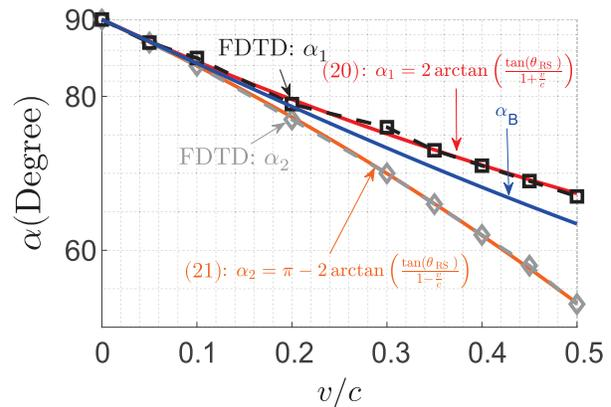
Fig. 17. Simulated reflection angles for inclined PRS moving with speed  $v$  toward  $\pm x$  directions, with  $\theta_{\text{PRS}} = 45^\circ$ . Bradley's aberration angle  $\alpha_B$  is also plotted for comparison.
