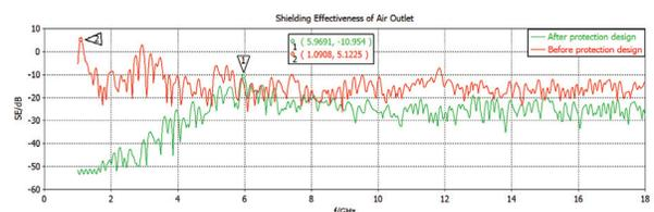
Fig. 19. Shielding effectiveness of the air outlet after protection design.
