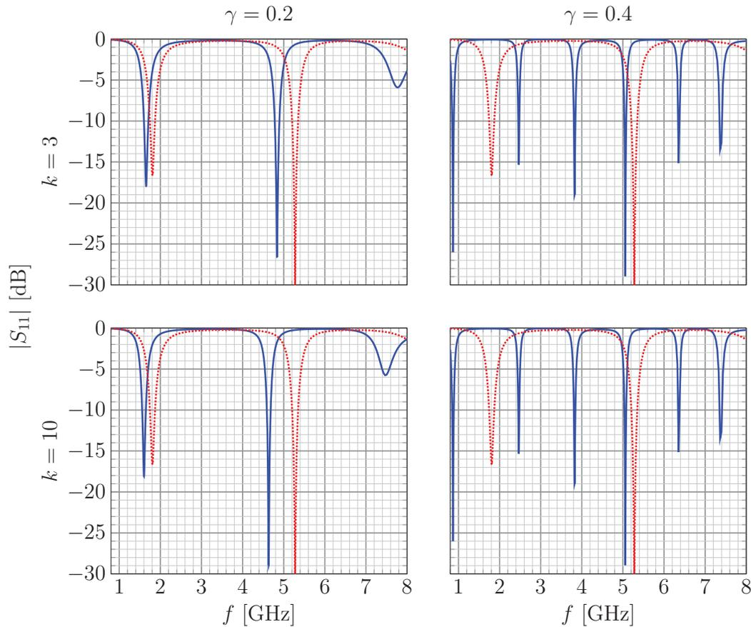
Fig. 3.  $|S_{11}|$  versus the frequency  $f$  for varying  $k$  and  $\gamma$ . (—) and (.....) indicates the prefractal and the reference bend wire antenna corresponding to  $k = 1$  case, respectively.
