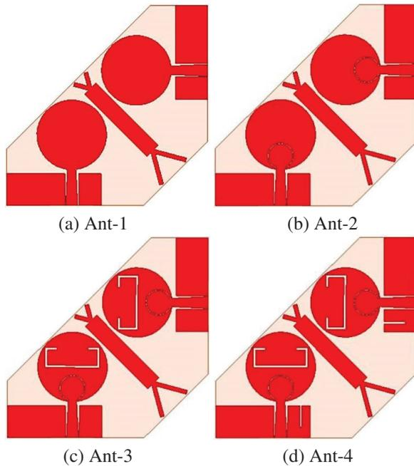
Fig. 2. Design process of notched band MIMO antenna.
