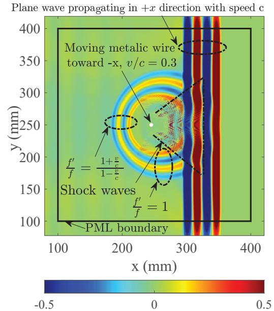
Fig. 20. Electric field distribution for a metallic wire moving toward a plane wave source in  $-x$  direction with  $\frac{v}{c} = 0.3$ . The plane wave is propagating in  $+x$  direction with speed  $c$ .
