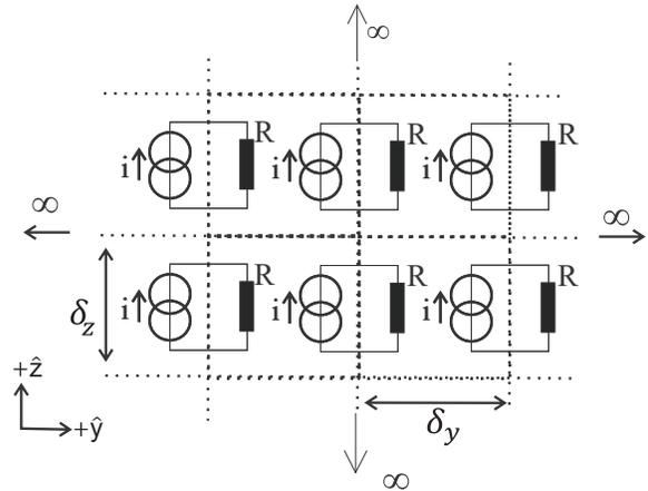
Fig. 5. Model of a plane wave source used in FDTD.
