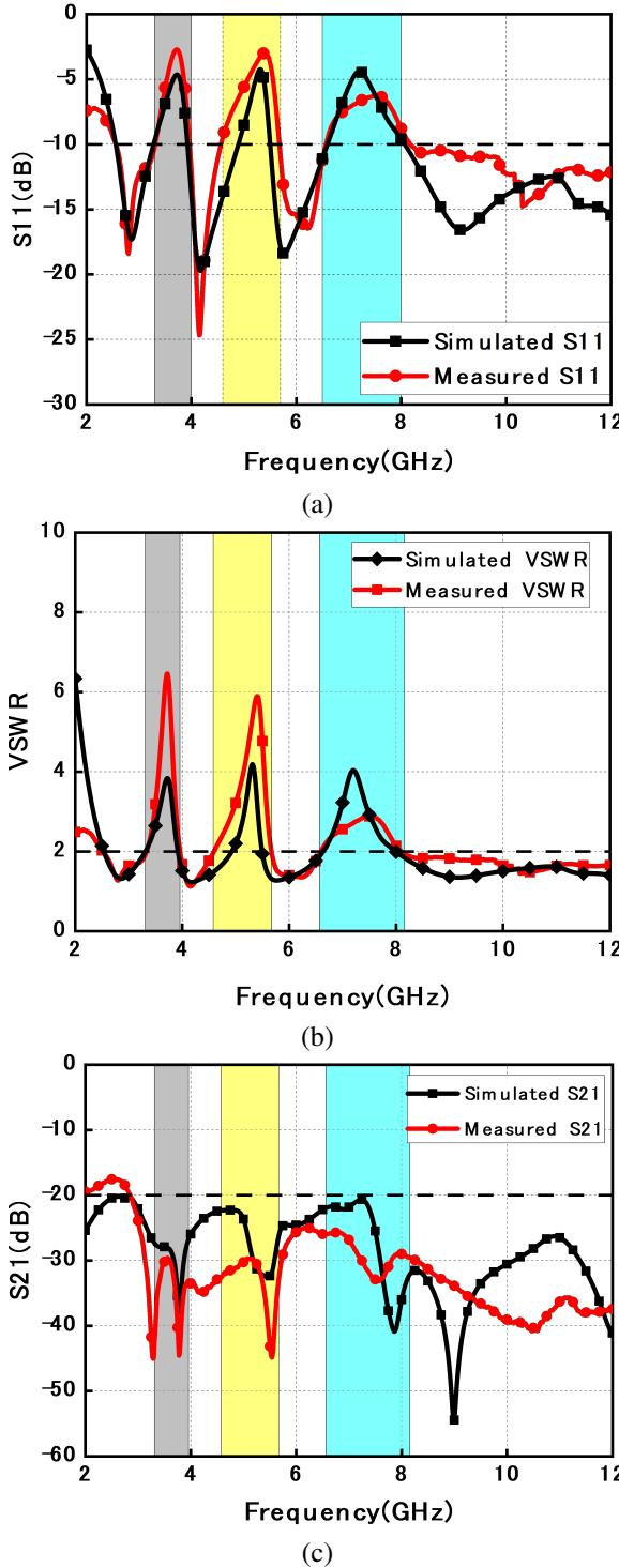
Fig. 10. Comparisons between simulated and measured values of S-parameters: (a)  $S_{11}$ , (b) VSWR, (c)  $S_{21}$ .
