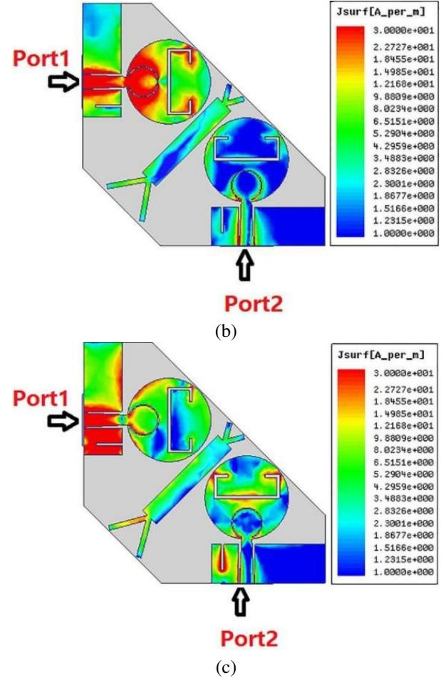
Fig. 9. Simulated surface current distribution when Port 1 acts as the exciter: (a) 3.4 GHz, (b) 5.25 GHz, and (c) 7.5 GHz.
