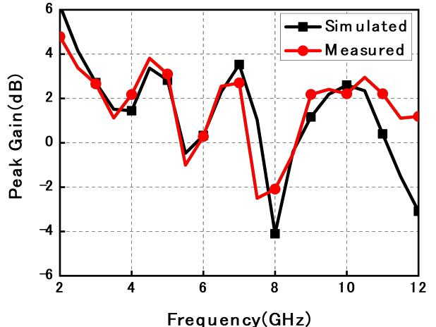
Fig. 14. Simulated and measured gain of MIMO antenna.
