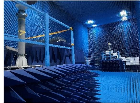
Fig. 11. Antenna far field measurement setup.
