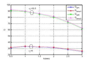
Fig. 7. The variation of Q-factor of surface wave with *h* for two different  $\varepsilon_r$  and R = 7mm.
