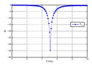
Fig. 10. Return loss as function of frequency.
