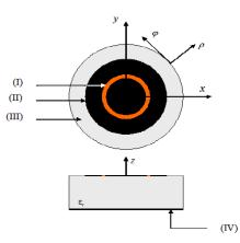
Fig. 4. Configuration of the circular patch: (I) excitation ring, (II) circular patch, (III) dielectric, (IV) ground plane.
