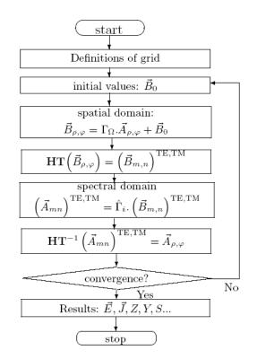
Fig. 3. The WCIP algorithm.
