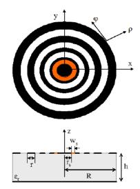
Fig. 1. Multi-slits antenna design.
