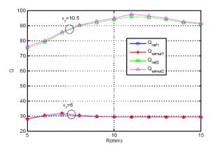
Fig. 8. The variation of Q-factor of surface wave with *R* for two different  $\varepsilon_r$  and h = 1.27mm.
