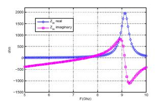
Fig. 11. Real and imaginary parts of input impedance of antenna with two slits.
