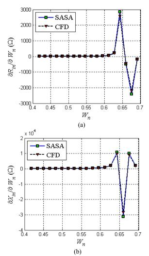
Fig. 7. Sensitivity of the input impedance with respect to  $W_n$  at  $L_n = 0.48$ : (a) resistance derivative; (b) reactance derivative.
