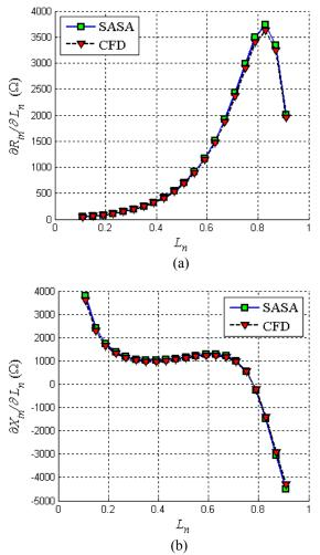
Fig. 3. Sensitivity of the input impedance of the Yagi-Uda antenna with respect to the normalized length of the driving element: (a) resistance derivative; (b) reactance derivative.
