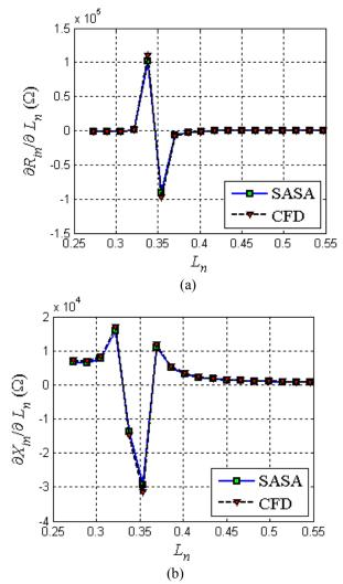
Fig. 6. Sensitivity of the input impedance with respect to  $L_n$  at  $W_n = 0.66$ : (a) resistance derivative; (b) reactance derivative.
