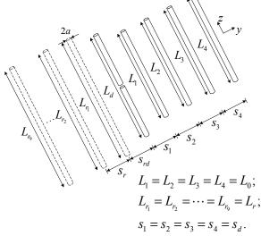
Fig. 2. Six-element Yagi-Uda antenna.
