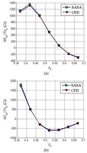
Fig. 4. Sensitivity of the input impedance of the Yagi-Uda antenna with respect to the distance between the driving element and the reflector: (a) resistance derivative; (b) reactance derivative.
