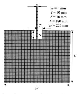
Fig. 5. Library structure of a planar patch.
