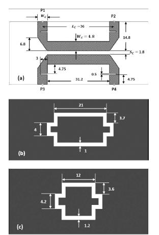
Fig. 16. Geometric dimension of the fabricated meandered DGS couplers 2 and 3. (a) The top layer geometry used for both couplers. (b) DGS geometry of coupler 2. (c) DGS geometry of coupler 3. All dimensions are in mm.
