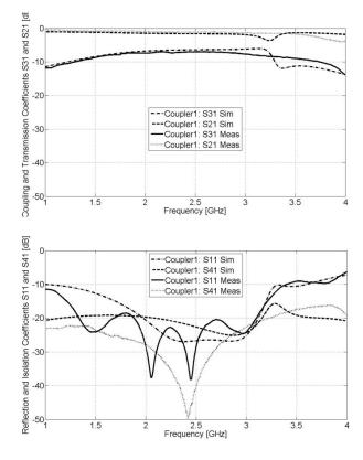
Fig. 15. Simulated and measured S-parameters of DGS coupler (coupler-1).
