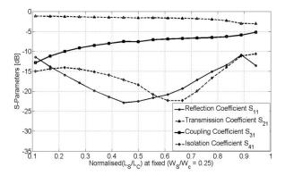
Fig. 11. Variation of S-parameters of the modified coupler against  $(L_S / L_C)$  at fixed  $(W_S / W_C = 1/4)$ . The notch dimensions are 4 mm x 0.5 mm.
