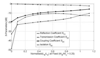
Fig. 4. The S-parameters against normalized ( $L_S / L_C$ ) at fixed ratio ( $W_S / W_C = 1/4$ ).
