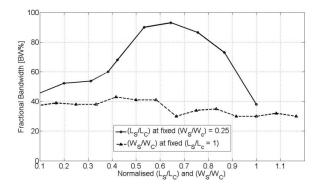
Fig. 6. Fractional bandwidth (B%) against  $(L_S / L_C)$  and  $(W_S / W_C)$  at fixed ratios of  $(W_S / W_C = 1/4)$  and  $(L_S / L_C = 1)$  respectively.
