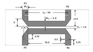
Fig. 10. Geometry of the modified initial coupler with a notch in feed arms. All dimensions are in mm.
