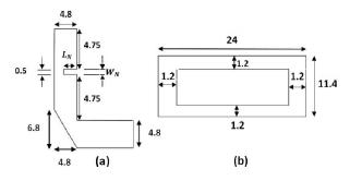
Fig. 8. Geometry of the notch length  $(L_N)$  and associated DGS of the coupler.
