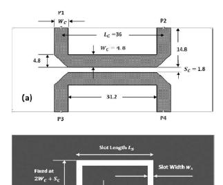
Fig. 1. Initial microstrip coupler with DGS. All dimensions are in mm. (a) Geometry of the -20 dB coupler. (b) DGS rectangular slot loop.
