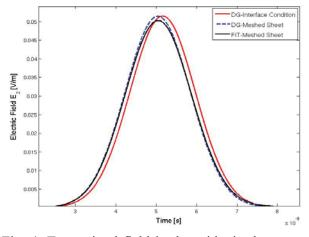
Fig. 4. Transmitted field in the midpoint between the sheets.
