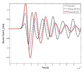
Fig. 10. Electric field in the center of the cavity.
