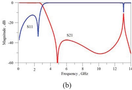
Fig. 8. The combination of two modified Hairpin resonators (a) layout and (b) simulation results.
