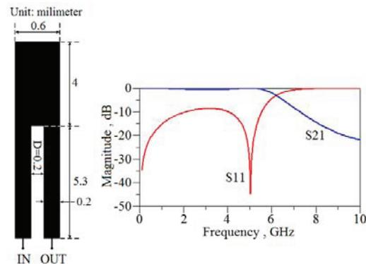
Fig. 1. Conventional hairpin resonator and its S-parameters results.
