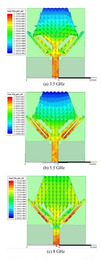
Fig. 2. Simulated surface current on the radiation patch: (a) 3.5 GHz, (b) 5.5 GHz, and (c) 8 GHz.
