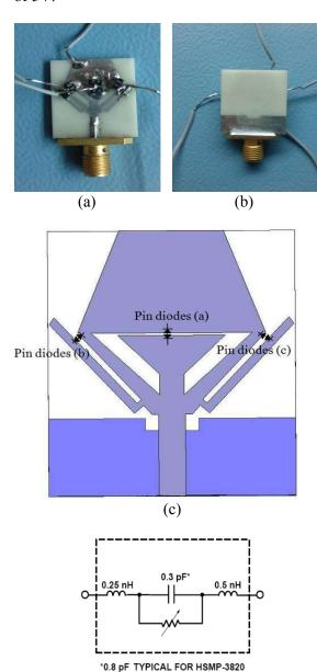
Fig. 5. (a) Photograph of antenna with PIN switching diodes, (b) back plane of the antenna, (c) location of the PIN diodes in the patch antenna, and (d) equivalent circuit of PIN diode (HSMP 3820).
