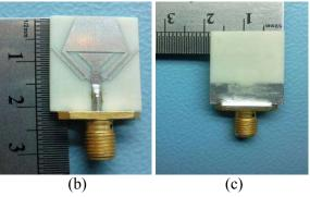
Fig. 1. (a) Geometry of proposed antenna, (b) top view of the proposed UWB antenna, and (c) bottom view of the antenna with ground plane.
