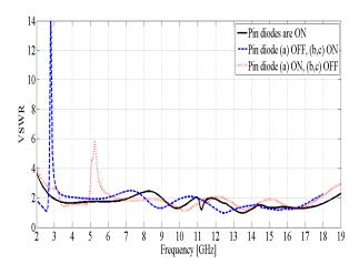
Fig. 6. Simulated VSWR for the antenna with and without band-notched function.
