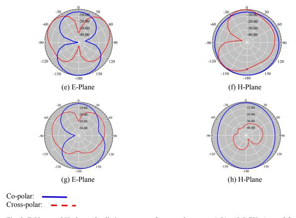
Fig. 9. E-Plane and H-plane of radiation patterns of proposed antenna: (a,b) at 3.5 GHz (central frequency of first notched band), (c,d) at 4.5 GHz (antenna operating frequency between first and second notched band), (e,f) at 5.5 GHz (central frequency of second notched band), and (g,h) at 9 GHz.
