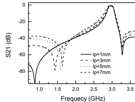
Fig. 10. Simulated scattering parameters of the filter B for four values of  $l_p$ .
