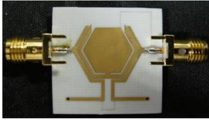
Fig. 11. Photograph of the fabricated filter B. Geometric parameters of the filters are  $w = 1$ ,  $r_2 = 5$ ,  $r_3 = 8$ ,  $l_2 = 11.55$ ,  $l_3 = 8$ ,  $l_p = 4$ ,  $s_2 = 1.5$  and  $s = 0.18$ . All are in mm.
