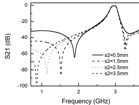
Fig. 9. Simulated scattering parameters of the filter B for four values of  $s_2$ .
