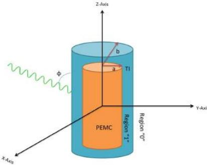
Fig. 1. PEMC Cylinder coated with topological insulator.
