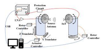
Fig. 2. Schematic for the designed antenna pattern measurement system [4].
