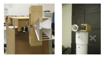
Fig. 4. Source fixture with source horn (left) and AUT fixture with mounted dipole antenna (right).
