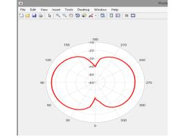
Fig. 1. The measured y-z plane pattern cut of a z-directed half-wavelength dipole antenna [4].
