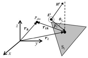
Fig. 1. Position vectors, observation point  $P_{obs}$ , propagation vector  $\hat{p}_i$ , angle of incidence  $\theta_i$ , incident electric and magnetic fields, and facet  $S_i$ .
