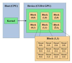
Fig. 2. CUDA Threading model.
