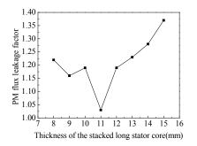
Fig. 9. PM flux leakage factor versus axial thickness of the stacked long stator core.
