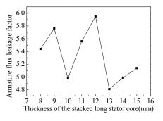
Fig. 5. Armature flux leakage factor versus axial thickness of the stacked long stator core.
