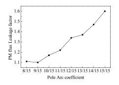
Fig. 10. The PM flux leakage factor versus the pole arc coefficient.
