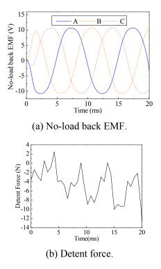
Fig. 12. No-load performance of circumference 3-phase structure.
