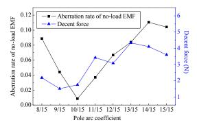
Fig. 15. The decent force and aberration rate of noload EMF versus pole arc coefficient.
