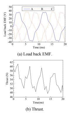
Fig. 14. Load performance of the circumference 3-phase structure.
