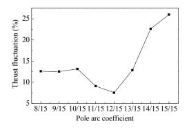
Fig. 17. Thrust fluctuation versus pole arc coefficient.
