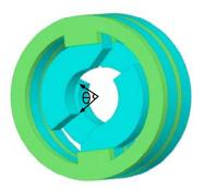
Fig. 24. Overlapping cross-sectional angle of adjacent stator core.
