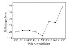
Fig. 7. PM flux leakage factor versus pole arc coefficient.
