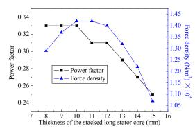
Fig. 19. Power factor and force density versus axial thickness of the stacked long stator core.
