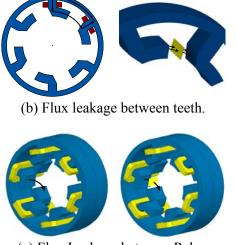
(c) Flux Leakage between Poles.
