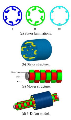
Fig. 2. Circumferential 3-phase structure.
