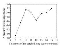
Fig. 8. Armature flux leakage factor versus axial thickness of the stacked long stator core.
