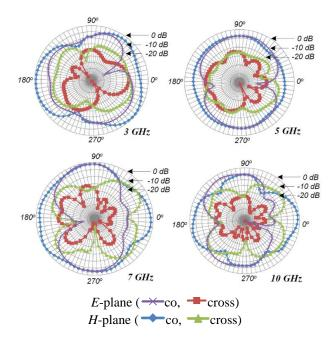
Fig. 9. Measured *E*-plane (x-z) and *H*-plane (y-z) radiation patterns of the proposed fractal antenna at various spot frequencies.
