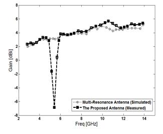
Fig. 12. Measured and simulated maximum gains for the proposed antenna.
