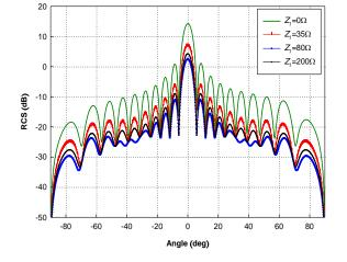
Fig. 5. Dependence of RCS pattern of a 25element unequal-length dipole array on the terminal impedance.
