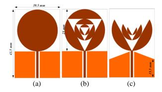
Fig. 1. Steps required to create the antenna structure.
