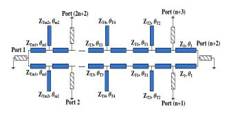
Fig. 3. Configurations of the proposed harmonic suppressed BPPD.
