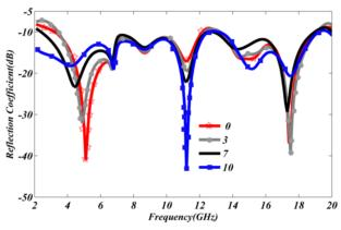
Fig. 6. Simulated reflection-coefficient plot for different values of  $\alpha$ .
