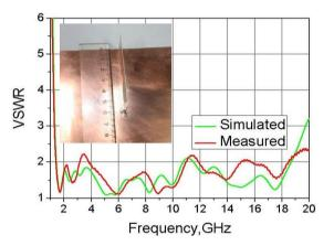
Fig. 2. Simulated and measured VSWR for the proposed antenna.
