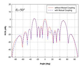
Fig. 4. Scanned ( $\theta_s$ =50°) RCS patterns of 20element unequal length linear dipole array, with and without mutual coupling effect.
