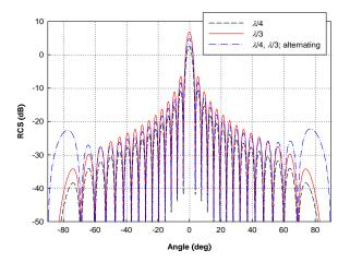
Fig. 3. Broadside RCS of equal and unequal length series-fed dipole array.
