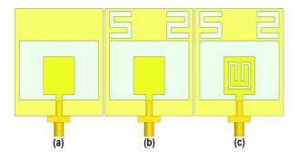
Fig. 2. (a) Ordinary slot antenna, (b) antenna with a pair of S-shaped slots in the ground plane, and (c) the proposed slot antenna.
