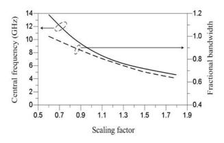
Fig. 11. The central frequency and fractional bandwidth of the basic resonator as a function of the scaling factor.
