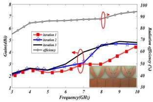
Fig. 10. Gain and efficiency plots for the three fractal iterations of the proposed antenna.
