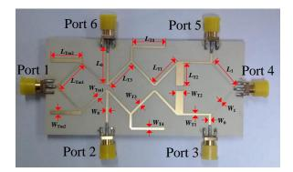
Fig. 7. Photograph of the fabricated proposed BPPD.
