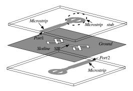
Fig. 1. Layout of the proposed microstrip-tomicrostrip vertical transition.
