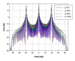
Fig. 8. Effect of varying the terminating impedances on the RCS pattern of 64-element unequal length parallel-in-echelon dipole array.
