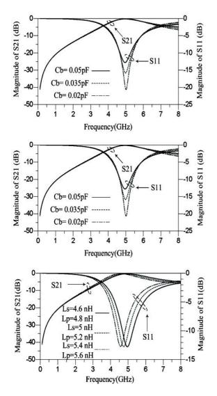
Fig. 7. Simulated results of the half-resonator model.
