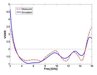
Fig. 7. Measured and simulated VSWR characteristics for the proposed antenna.
