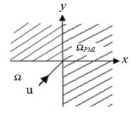
Fig. 2. The corner interface between  $\Omega$  and  $\Omega_{PML}$ .
