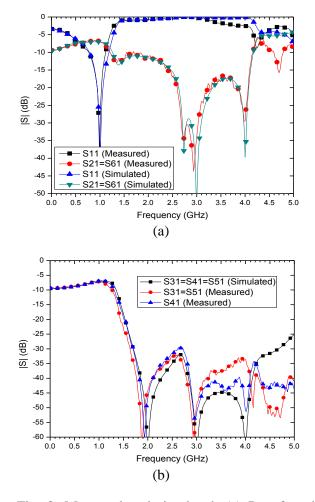
Fig. 8. Measured and simulated: (a) Port 2 and Port 6 have third harmonic suppression, and (b) Port 3, Port 4 and Port 5 have second, third and fourth enhanced harmonic suppression simultaneously.
