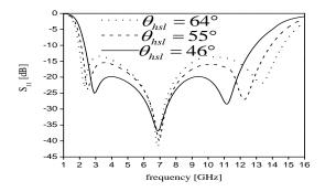
Fig. 5.  $S_{11}$  with different high-impedance slotline stub length  $\theta_{hsl}$ .
