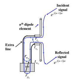
Fig. 1. The reflection and transmission coefficients till the phase-shifters.
