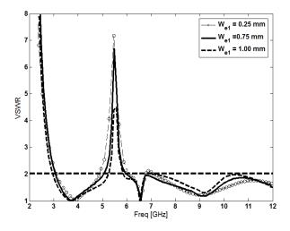
Fig. 7. Simulated VSWR characteristics for the proposed antenna with different values of We1.
