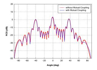
Fig. 7. Broadside RCS pattern of 16-element unequal length parallel-fed dipole array.
