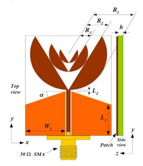
Fig. 2. The proposed antenna structure showing characterizing parameters.
