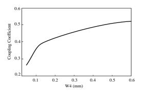
Fig. 4. Coupling coefficient of the proposed resonator versus the width of the central line.
