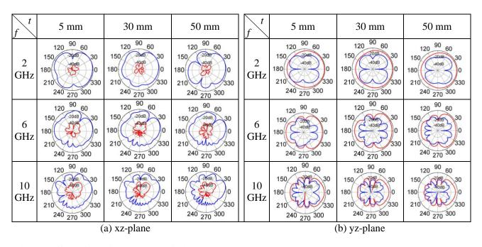
Fig. 12. Effect of the distance *t* on radiation pattern ( $--- E_{\phi}; ---- E_{\Theta}$ ).
