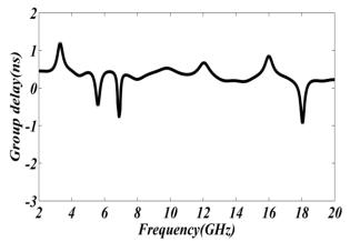
Fig. 11. Group delay plot of the antenna.
