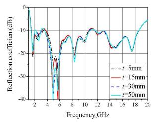
Fig. 11. Effect of distance t on reflection coefficient.
