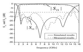
Fig. 7. Simulated and measured performance of the proposed transition.
