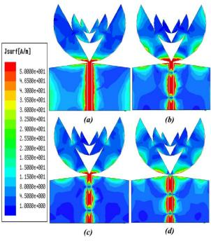
Fig. 8. Current distributions over the proposed antenna at: (a) 3 GHz, (b) 6 GHz, (c) 8 GHz, and (d) 10 GHz.
