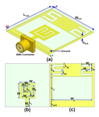
Fig. 1. Geometry of the proposed microstrip-fed slot antenna: (a) side view, (b) top layer, and (c) bottom layer.
