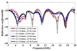
Fig. 5. Simulated reflection-coefficient plot for different values of  $L_1$  and  $L_2$ .
