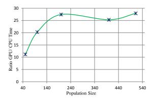
Fig. 10. Speedup: GA optimization GPU time/CPU time with population size.
