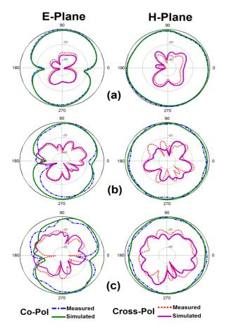
Fig. 6. Measured and simulated radiation patterns of the proposed antenna: (a) 5 GHz, (b) 9 GHz, and (c) 13 GHz.
