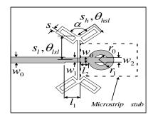
Fig. 2. Structure parameters of the proposed transition.
