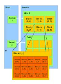
Fig. 3. The CUDA programming model.
