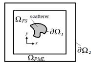
Fig. 4. The computational domain definition with the PML.
