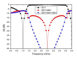
Fig. 5. The amplitude responses *S*-parameters of 5way third harmonic suppression BPPD.
