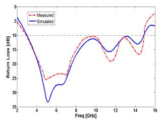
Fig. 8. Measured and simulated return loss characteristics for the proposed antenna.
