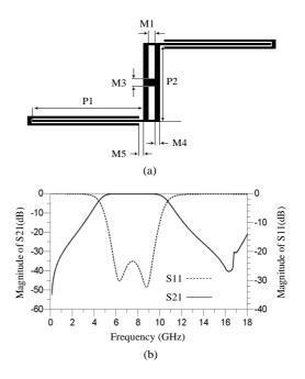
Fig. 2. Basic resonator with DMS: (a) layout, and (b) simulation results.
