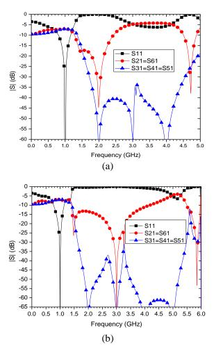
Fig. 6. The amplitude responses *S*-parameters of 5way enhanced harmonic suppression BPPDs: (a) Case 2, and (b) Case 3.
