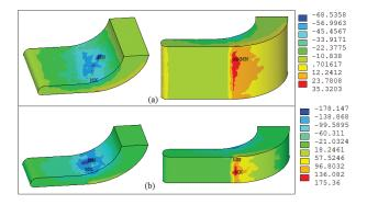
Fig. 7. Normal force distribution on the C-shape armature for  $X_C=Y_C=3$  cm: (a)  $h_a=4$  cm and (b)  $h_a=2$  cm.
