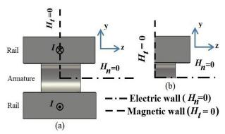
Fig. 4. Boundary conditions in rear view of railgun with C-shape armature.
