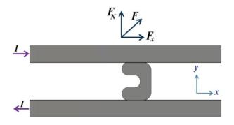
Fig. 3. The electromagnetic force and components.
