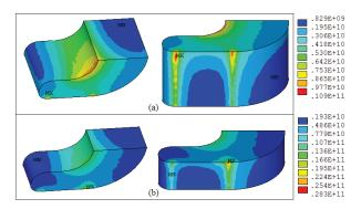
Fig. 8. Current density distribution on the C-shape armature for  $X_C=Y_C=2$  cm: (a)  $h_a=4$  cm and (b)  $h_a=2$  cm.
