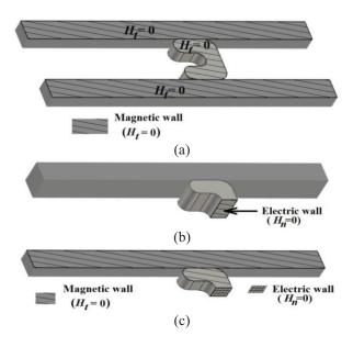
Fig. 5. 3D railgun: (a) half magnetic wall, (b) half electric wall, and (c) a quadrant of 3D railgun using magnetic and electric walls.
