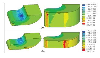
Fig. 9. Normal force distribution on the C-shape armature for  $X_C=Y_C=2$  cm: (a)  $h_a=4$  cm and (b)  $h_a=2$  cm.
