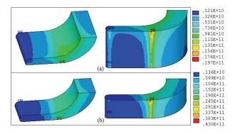
Fig. 6. Current density distribution on the C-shape armature for  $X_C=Y_C=3$  cm: (a)  $h_a=4$  cm and (b)  $h_a=2$  cm.
